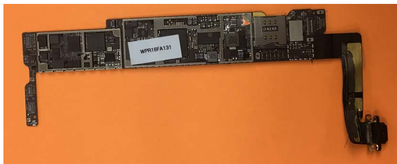
Figure 2. Internal printed circuit board removed from accident unit.
