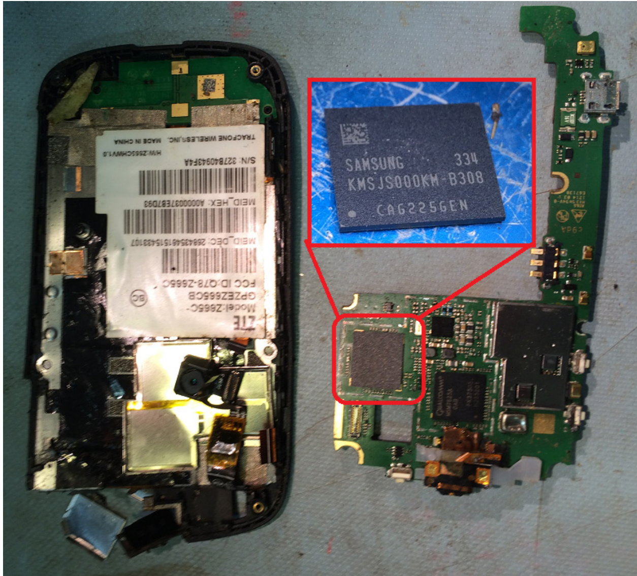
Figure 2. Internal inspection and non-volatile memory chip.
