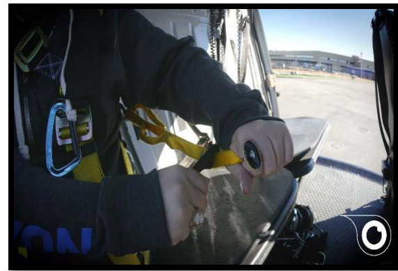
Figures 3-6: Screenshots from the FlyNYON safety video indicating the fitting of the harness system, release of the carabiner, location of the cutter and demonstrating how to cut the tether
