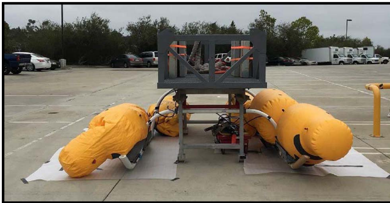
Figure 19: The inflated floats at the conclusion of the first inflation test
