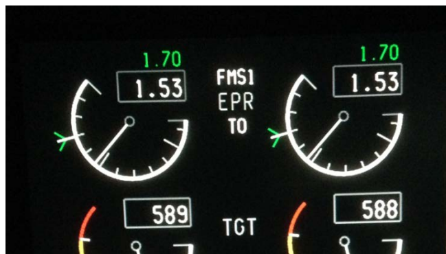
FIGURE 27 – SIMULATED STABILIZED ACCIDENT EPR VALUE NOT REACHING RATED EPR TARGET
