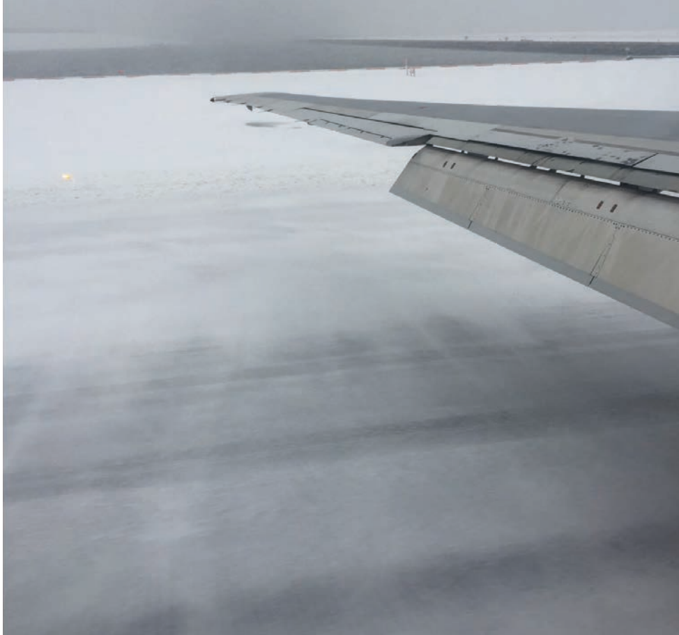
Figure 5: Passenger Photograph out of the left side window at the 500 foot runway marker. Note retracted spoiler panels.
