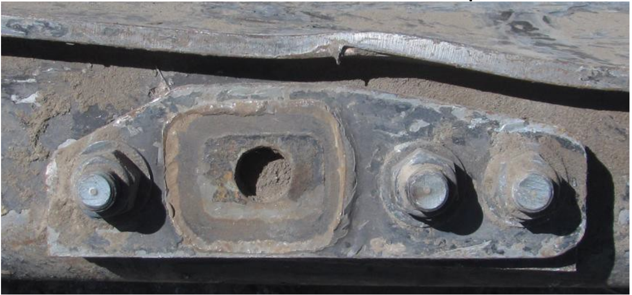
Figure 1. Fracture surface of Hyundai Rotem cab car 645 vertical tube weld.
