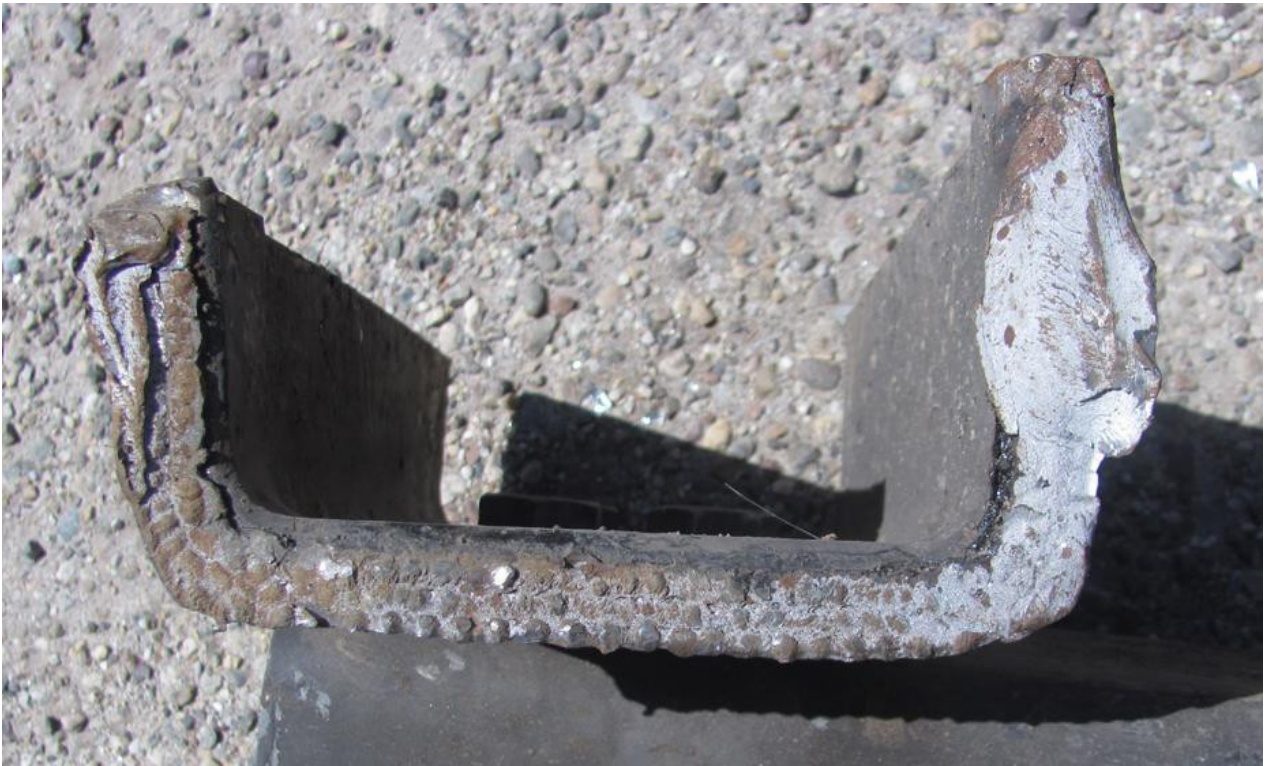
Figure 2. Fracture surface of the Hyundai Rotem cab car 645 left side horizontal channel weld.
