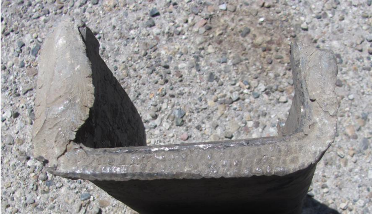
Figure 3. Fracture surface of the Hyundai Rotem cab car 645 right side horizontal channel weld.
