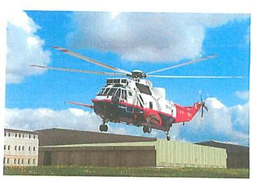
sea level and a typical summer temperature is around 35°C (95°F), so the British crews were flying at density altitudes of around 7,700 feet. They soon confirmed the payload improvement but were astounded by the speed increase. "We were expecting a fifteen knot premium but found that, in those conditions, the cruise had increased from 86 knots to a full 120 – nearly 35 knots more."
