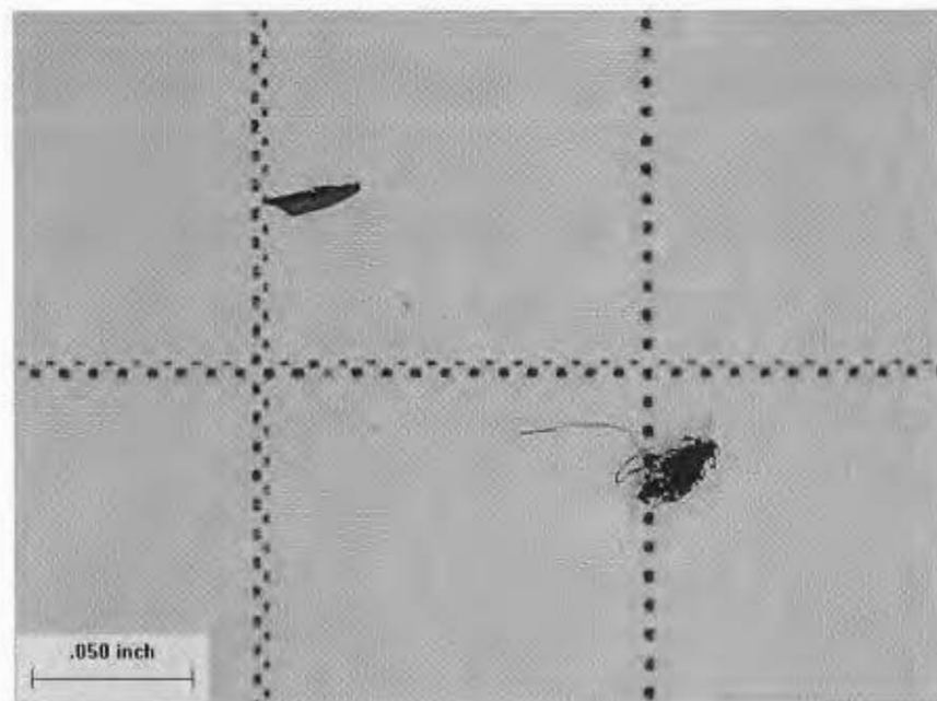
Figure 13: This photograph shows the 2 particles from the alcohol sample. Magnification: Approx. 20x
