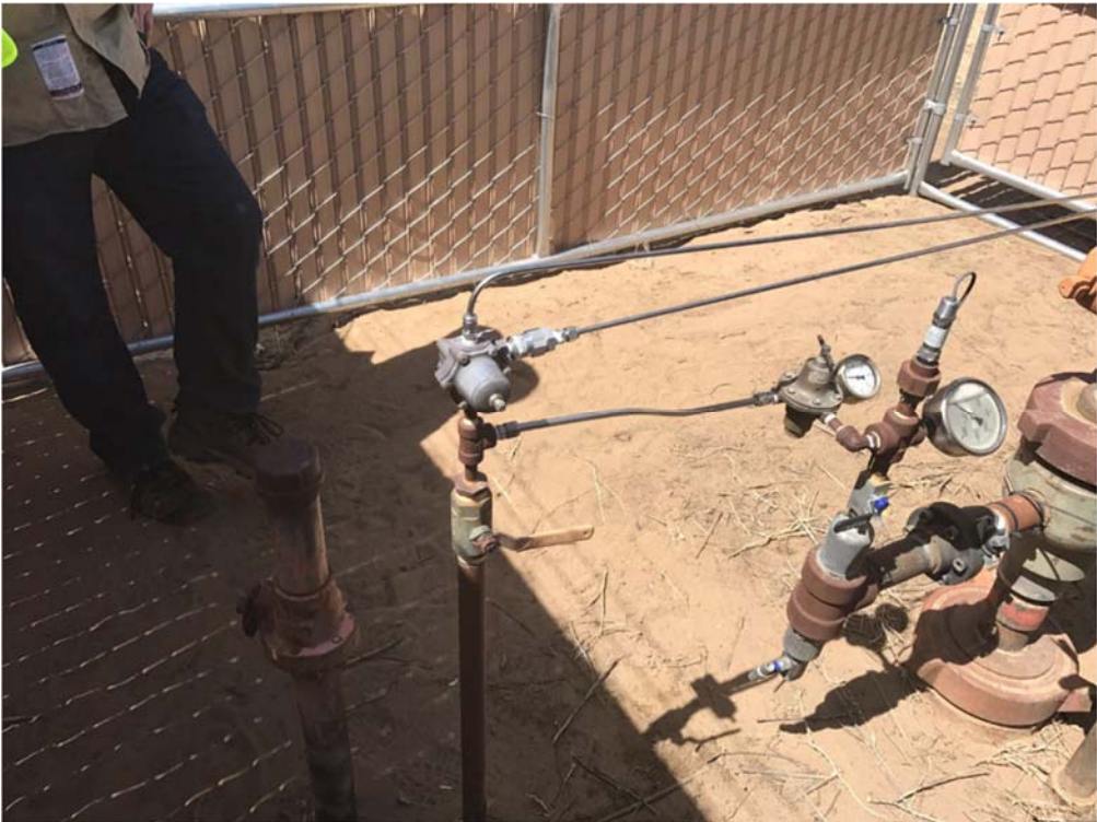
Figure 19: The Anadarko wellhead East of the exploded property with the 1’ line still connected, photo taken 4/18/2017
