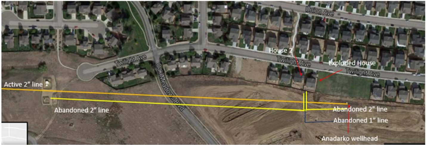
Figure 8: Sketch of active and abandoned pipeline going to the back of the yard (Note, the map is not official, not drawn to scale, but a pictorial description based on the trenched line)
