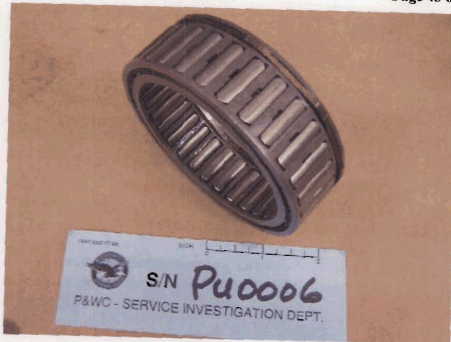
Photo no. 51 Closer view of the intact sprag clutch
