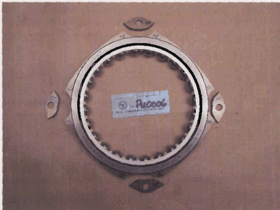
Photo no. 56 View of the four (4) fractured areas of the flanged No. 12 bearing outer ring
