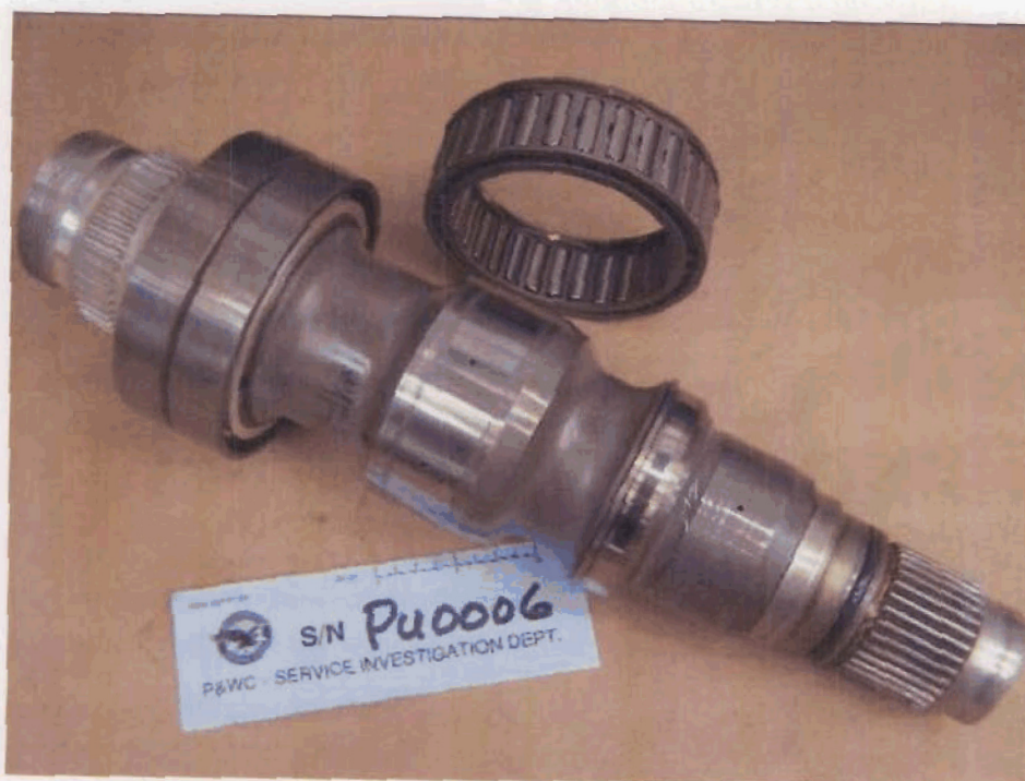
Photo no. 50 View of the intact RGB output shaft, sprag clutch & No. 14 duplex bearings
