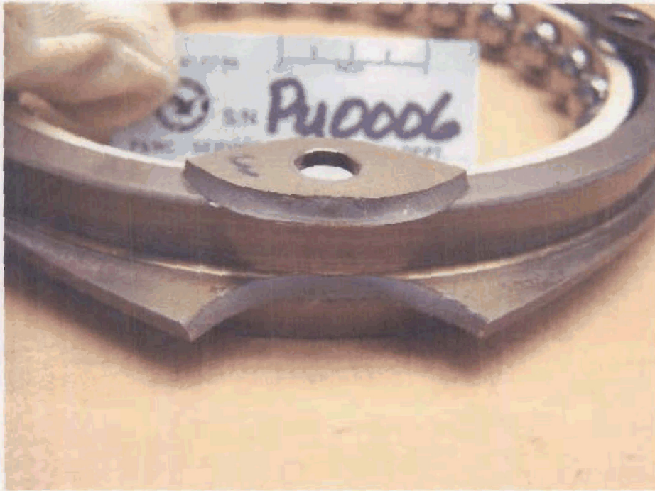
Photo no. 57 Detail view of the fracture surface of one of a fractured No. 12 bearing outer ring lug
