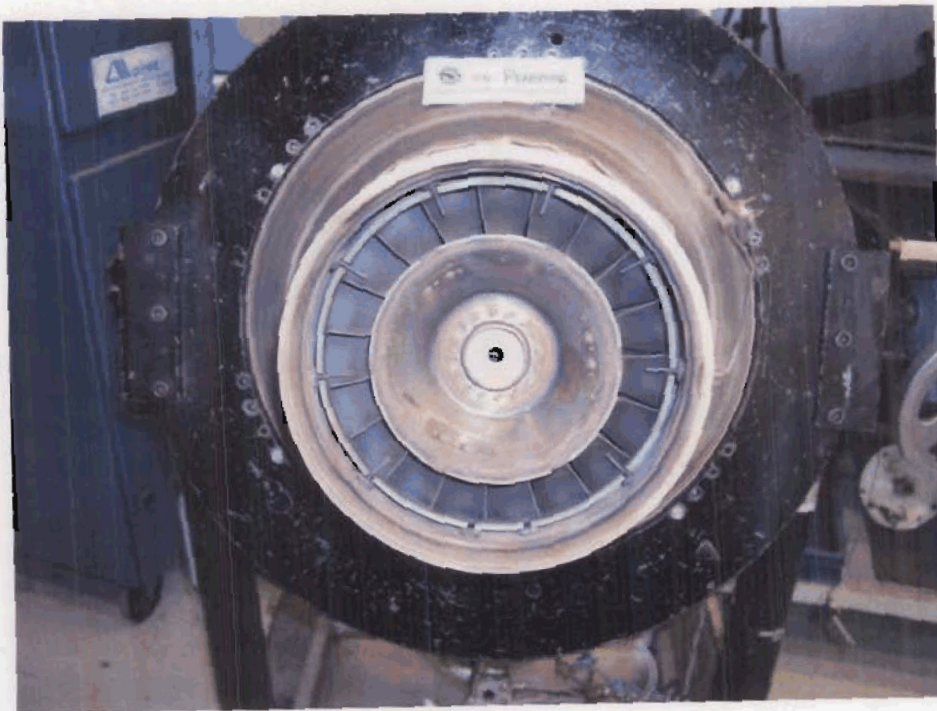
Photo no. 40 Leading edge view of the intact PT stator assembly
