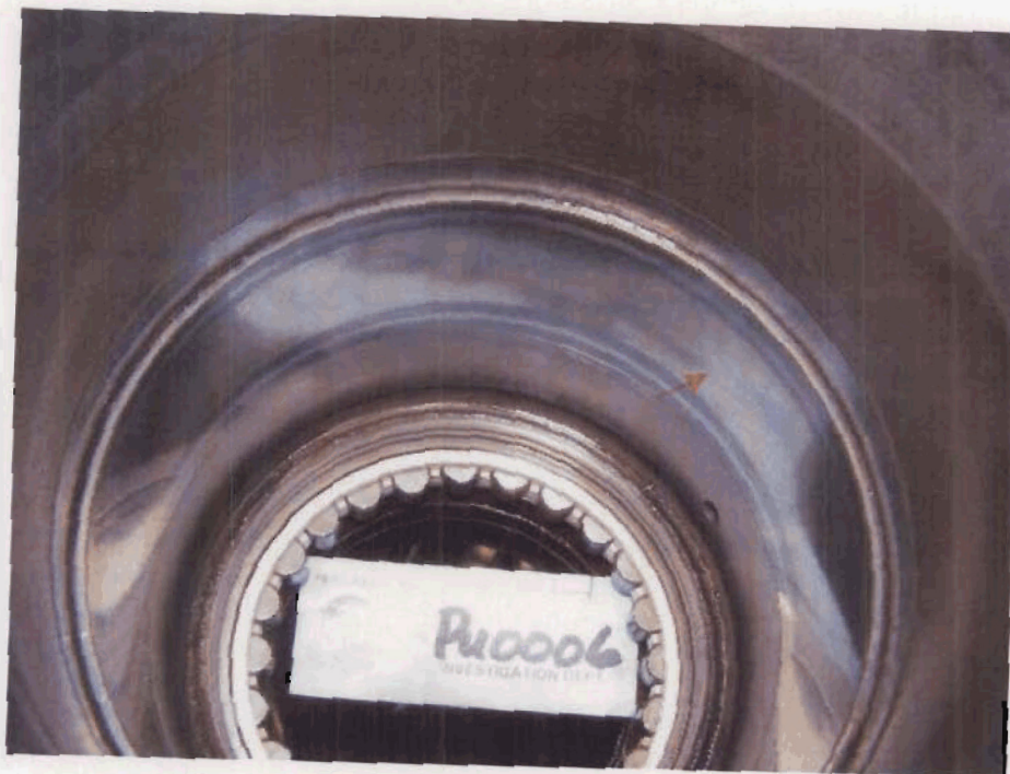
Photo no. 52 Inside view of the idler gear shows the intact runner (arrow) for the sprag clutch & the intact No. 15 roller bearing.
