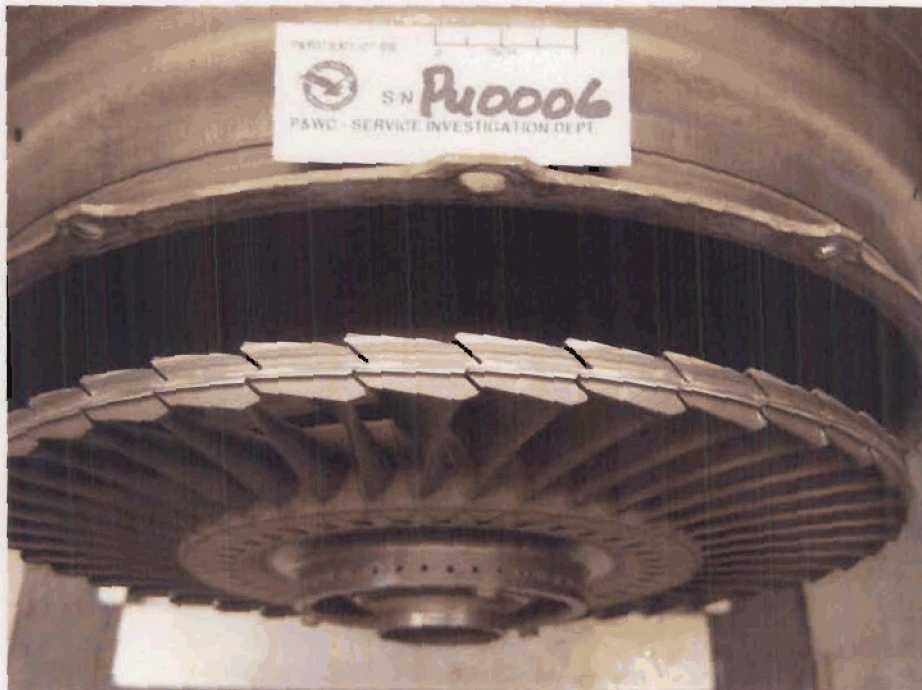
Photo no. 44 View of the PT blade shrouded tips show light rubs.
