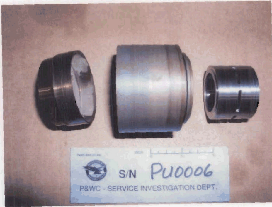
Photo no. 39 View of the compressor rotor air seals shows no impact rubbing damage to the OD's.
