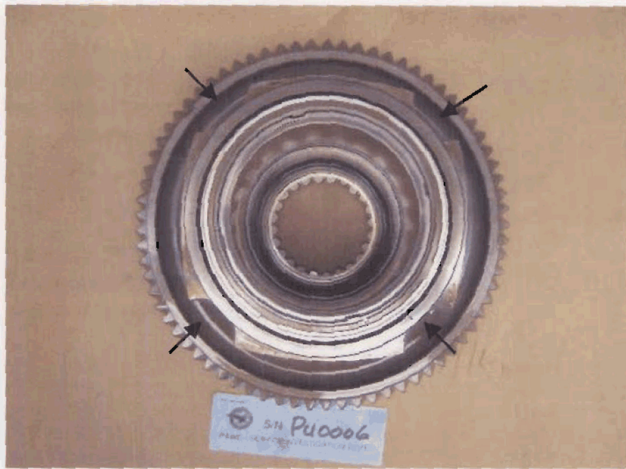
Photo no. 55 View of the No. 12 ball bearing attached to the idler gearshaft, which shows all four (4) fractures of the flanged outer ring.
