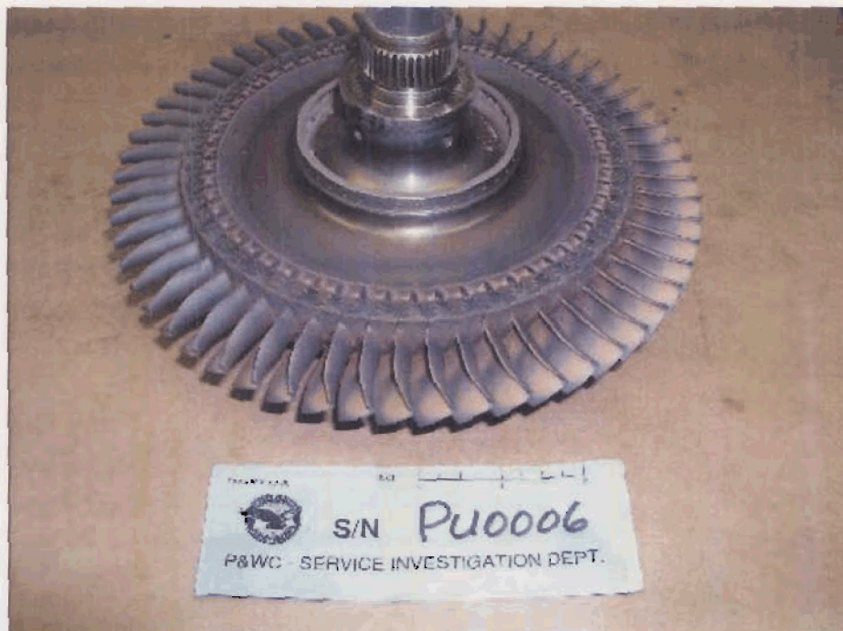
Photo no. 32 Leading edge view of the CT disc assembly
