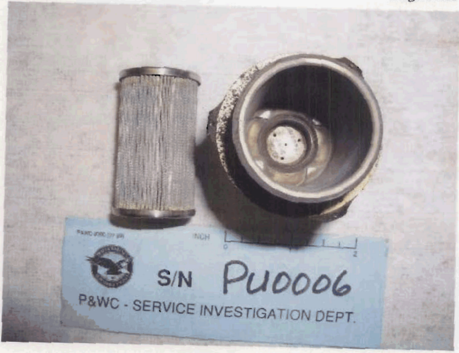
Photo no. 27 View of the P3 filter & the inside of the filter bowl being dry and clean
