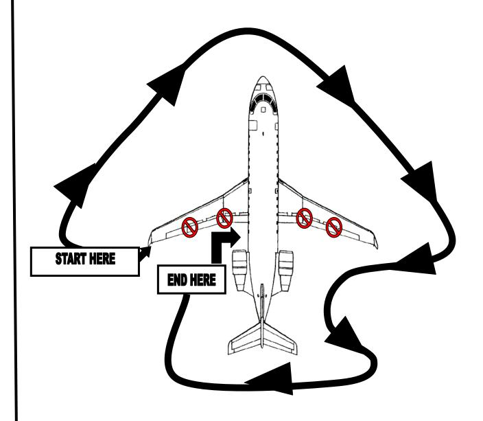
= Fluid application shall be leading edge to trailing edge.
