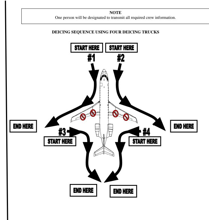
= Fluid application shall be leading edge to trailing edge.
