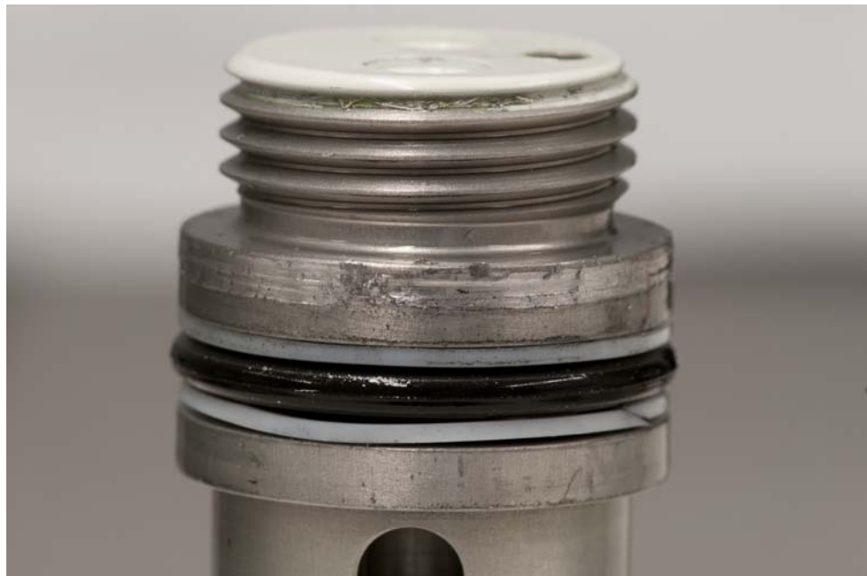
Photo 4, Galled Areas – Center Shaft OD – Upper End
