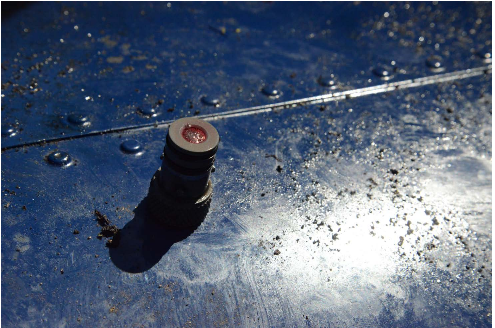
Photo 1 – View of the removed hydraulic system magnetic plug during recovery of the helicopter.
