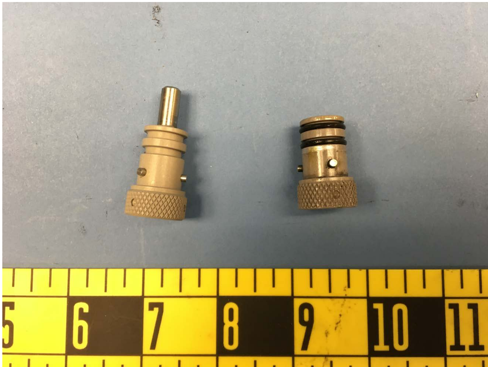
Photo 2 - Side view of the removed hydraulic system magnetic plug and an exemplar magnetic plug during the laboratory examination.
