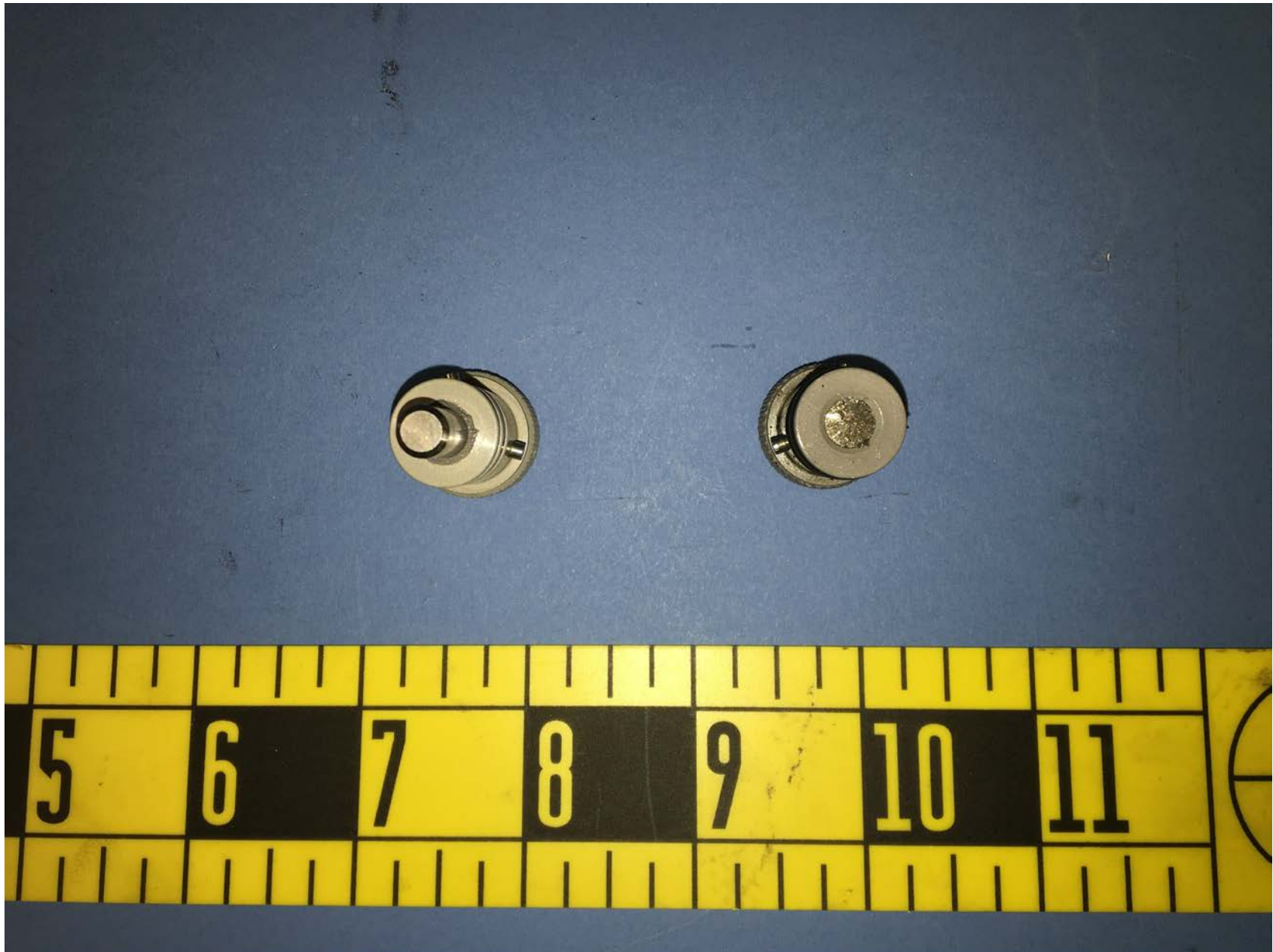
Photo 3 - Overhead view looking down at the removed hydraulic system magnetic plug and an exemplar magnetic plug during the laboratory examination.
