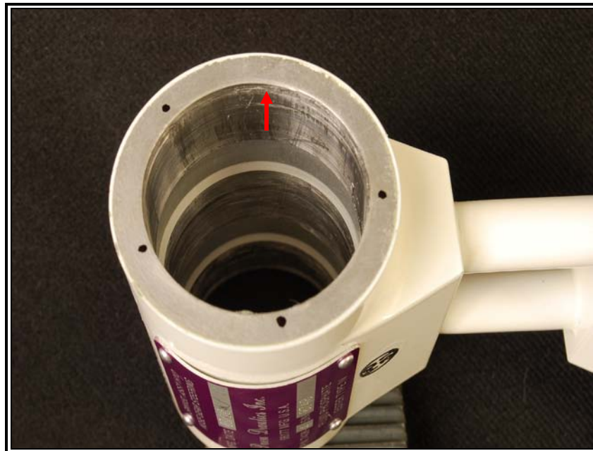
Figure 23: Photographs of the center housing outboard side showing wear (arrows)
