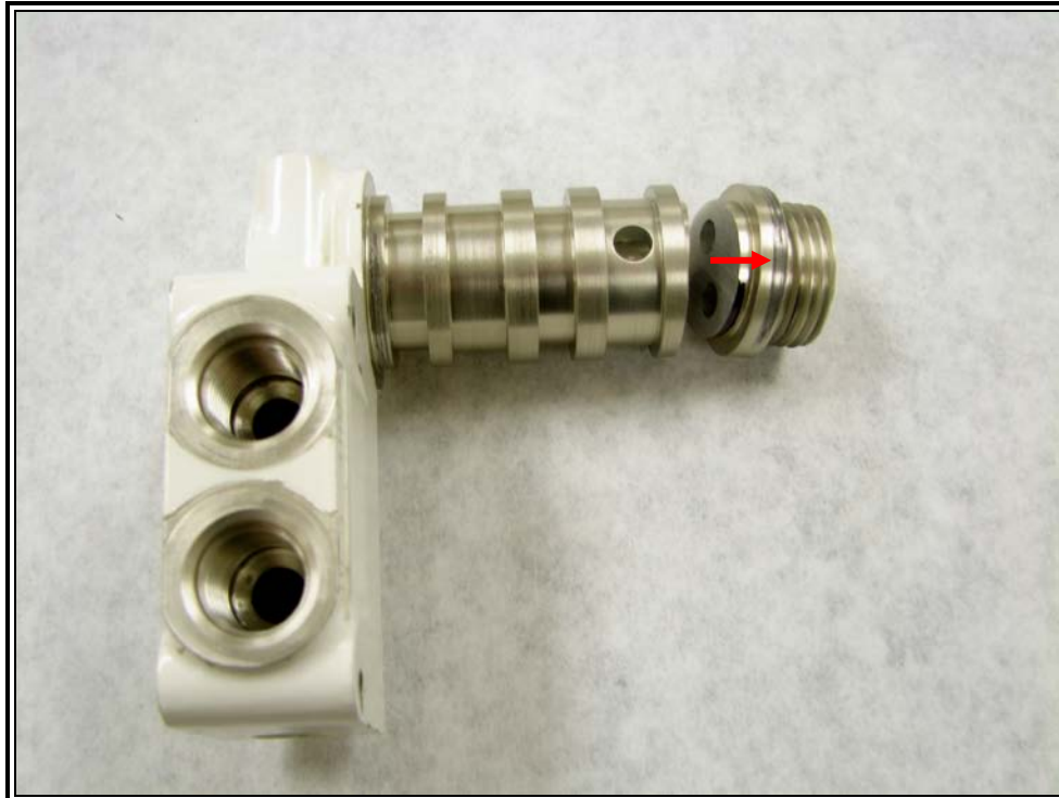
Figure 29: Photograph of the sectioned aft spool showing wear (arrow)
