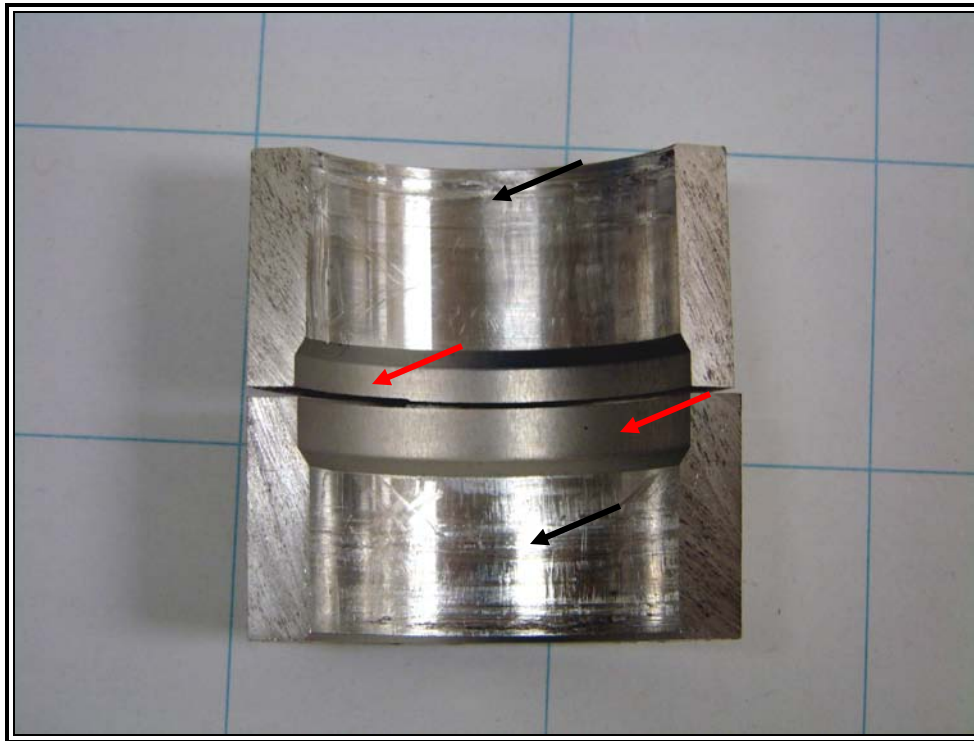
Figure 40: Photograph of a representative sectioned housing sample section showing the areas with anodizing (red arrows) and with no anodizing (black arrows) areas
