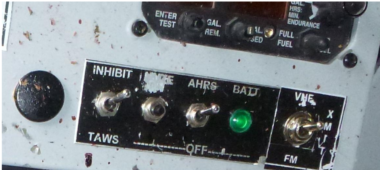
Figure 10. Photo of TAWS inhibit switch as found at accident site.
