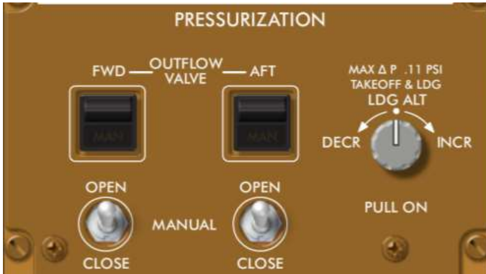
Figure 5: B-777 Pressurization Panel 35
