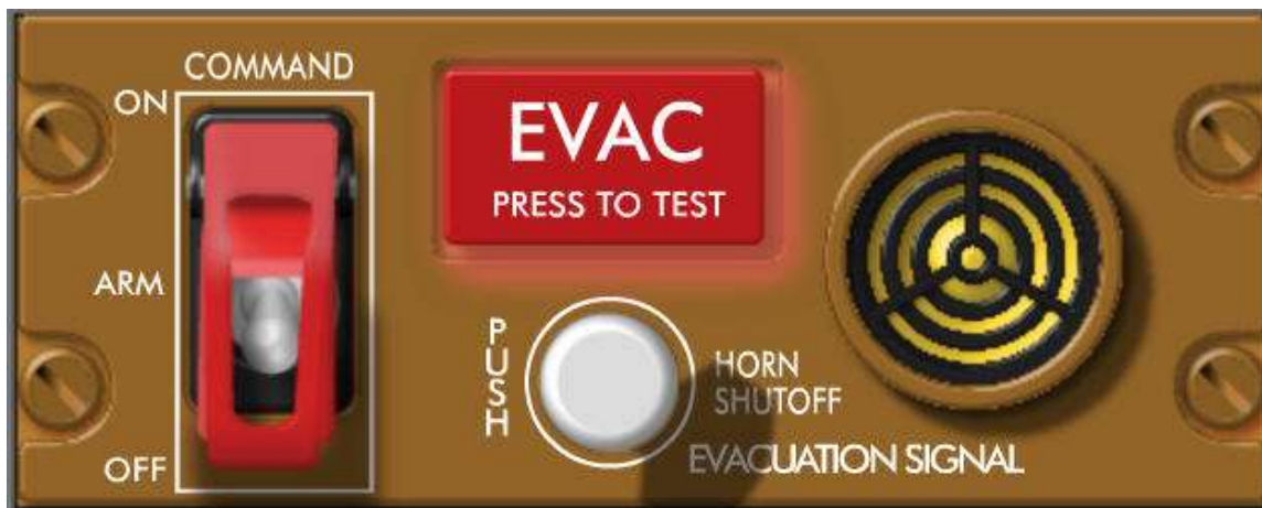
Figure 6: Emergency Evacuation Command Panel 36
