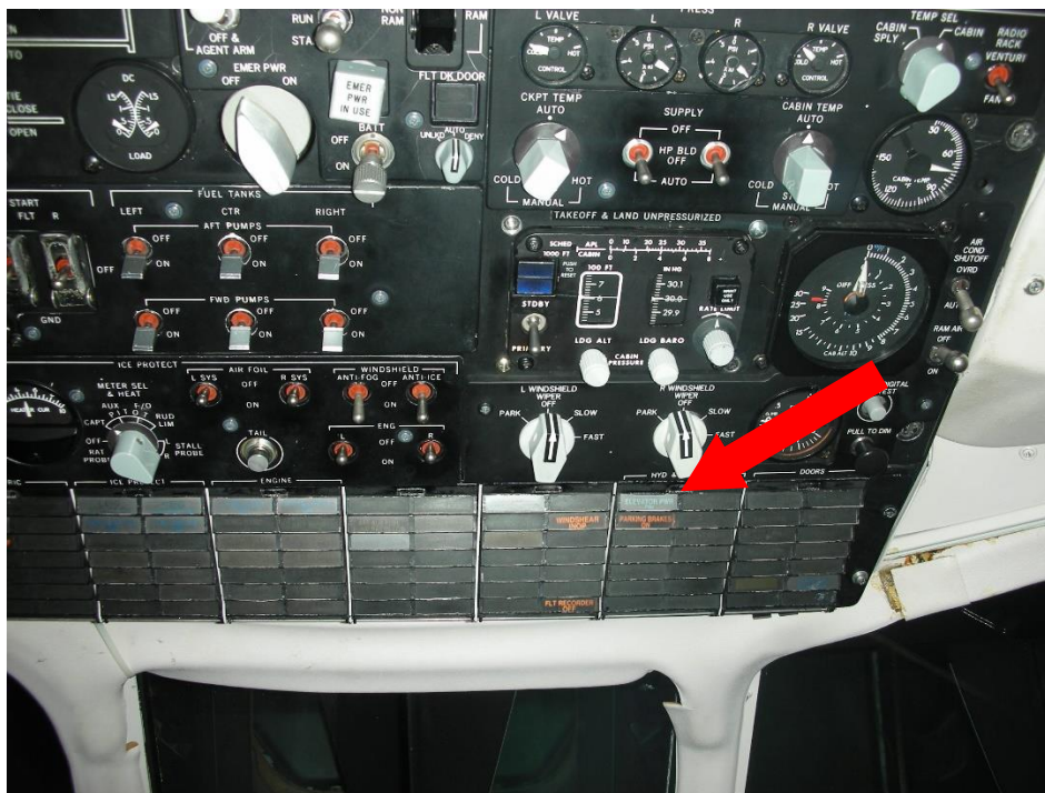
Photo 2: Overhead annunciator indications with control column full forward. “Elevator Pwr On” light indicated by arrow. 99
