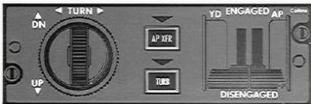
Figure 20: Vertical Speed toggle wheel (left) and Autopilot (and yaw damper – YD) engage panels (right). 147
