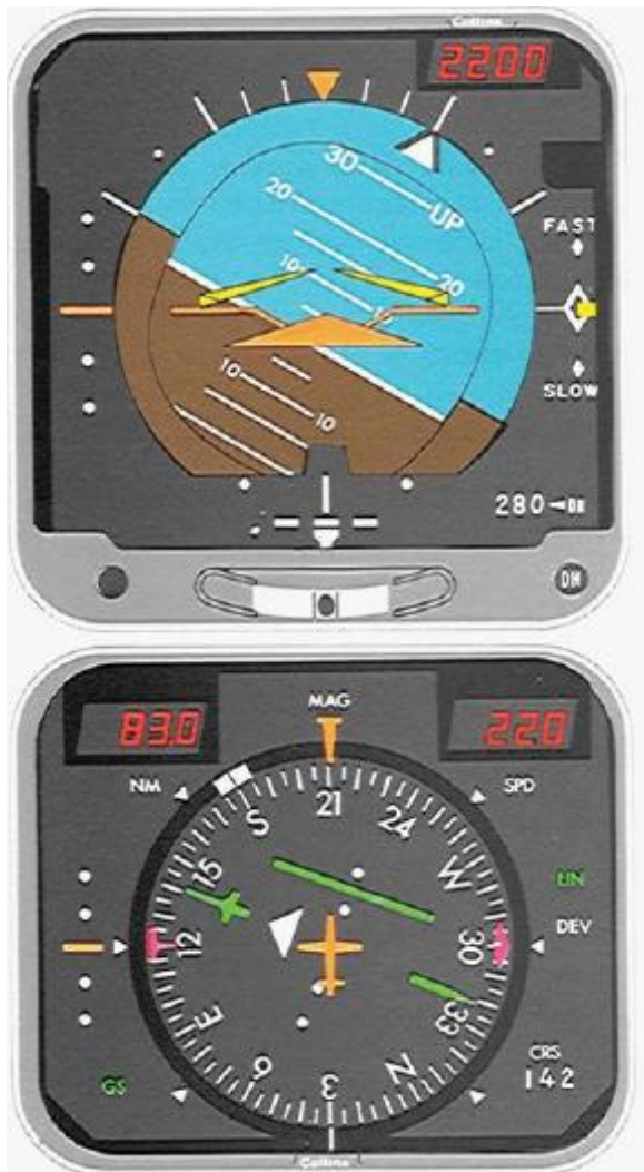
Figure 18: The Horizontal Situation Indicator (HSI) and the Attitude Director Indicator (ADI). 145
