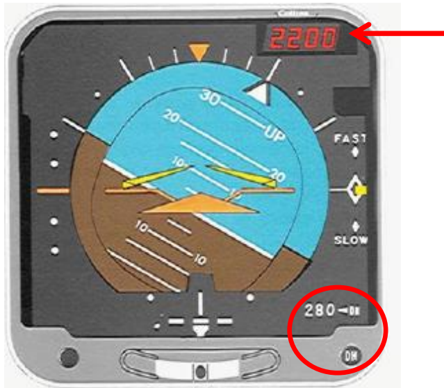
Figure 21: Decision Height (DH) select knob and amber DH annunciator (red circle) and radio altitude indicator (red arrow). 149
