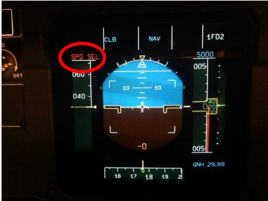
Photo 7: PFD after runway change with no V-speeds inserted in MCDU and SPD SEL on speed tape (indicated). 125
