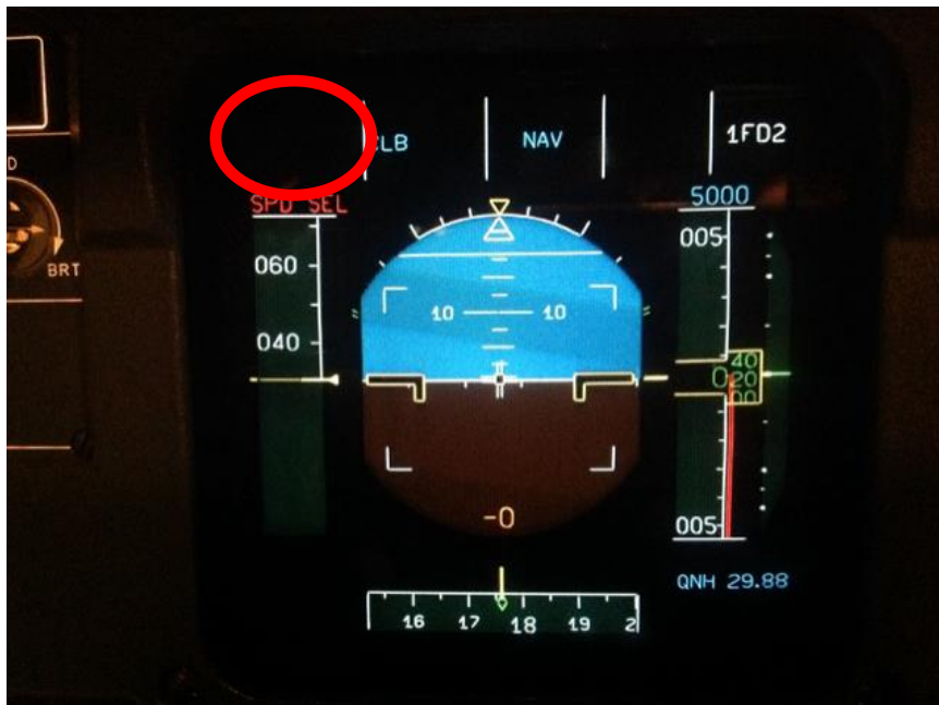
Photo 8: Autothrust column of the FMA (red circle). 126
