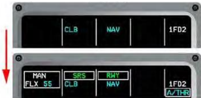
Photo 8: Sample FMA indications as FLEX thrust was set with FLEX temperature (55°) entered into the MCDU. 133
