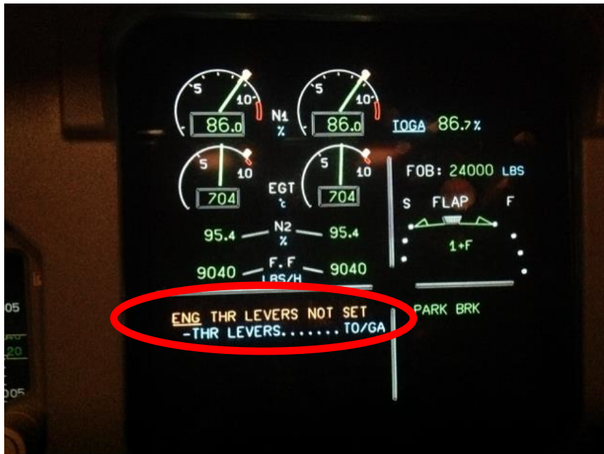
Photo 11: Upper ECAM when FLEX thrust set without a FLEX temperature, and ECAM message (indicated). 140
