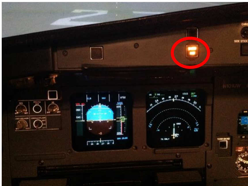
Photo 10: Forward displays with master caution (indicated) when FLEX thrust set without a FLEX temperature. 139
