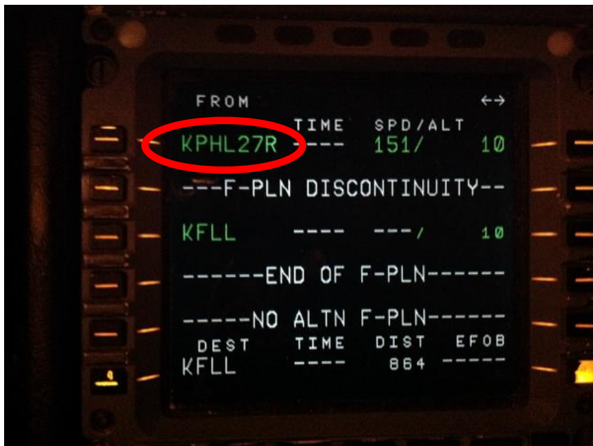
Photo 2: MCDU with PHL runway 27R (indicated) inserted in the flight plan page. 97
