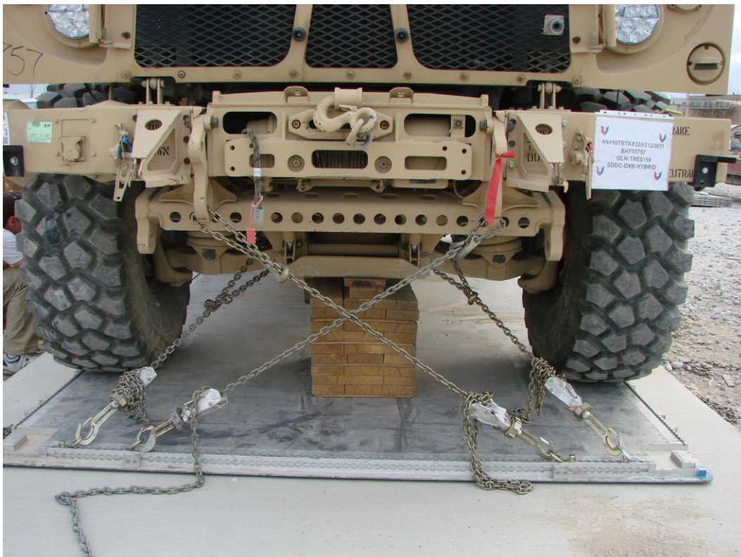
Photo 6: Photo of shoring demonstration of a 12-ton MATV (front view).
