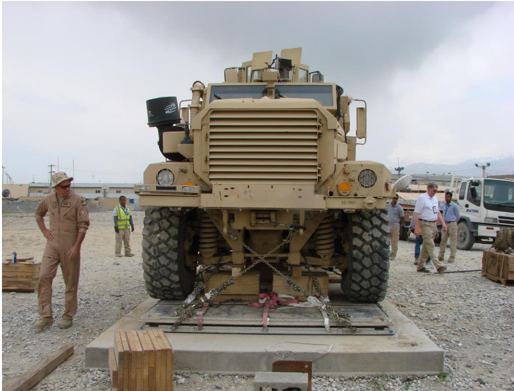
Photo 7: Photo of shoring demonstration of a 18-ton Cougar (front view).
