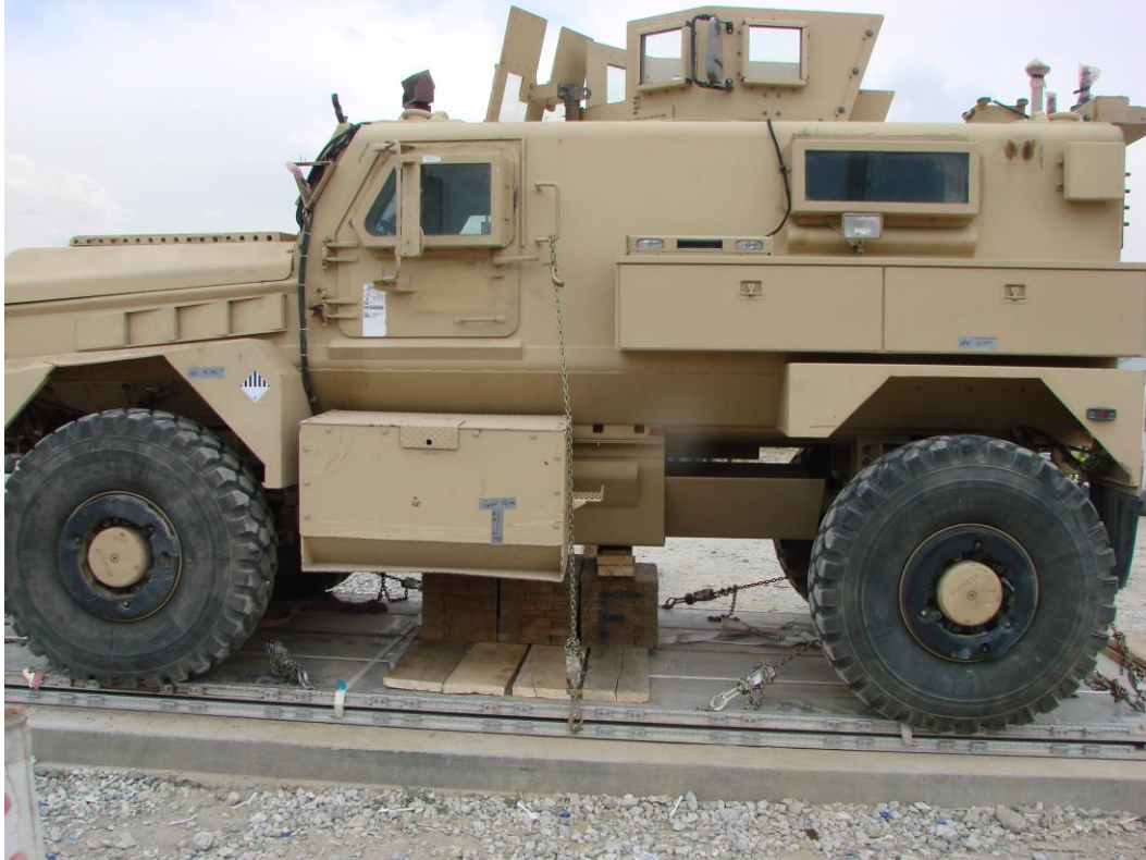
Photo 8: Photo of shoring demonstration of a 18-ton Cougar (side view).
