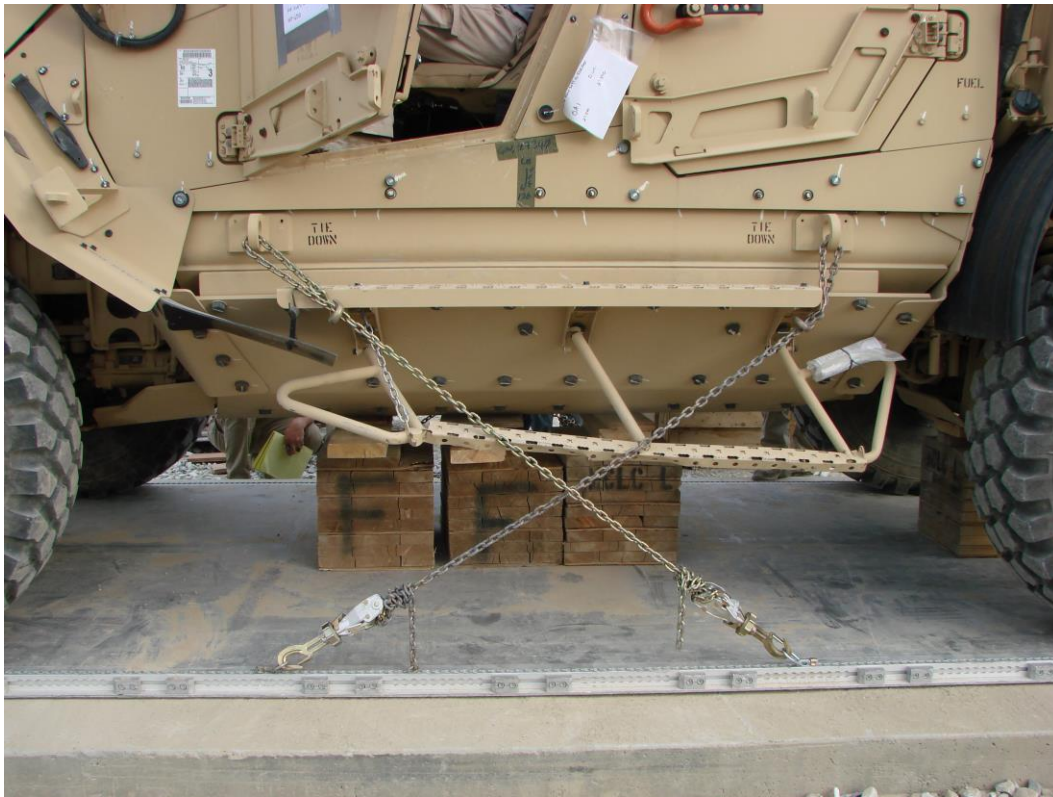
Photo 5: Photo of shoring demonstration of a 12-ton MATV (side view).
