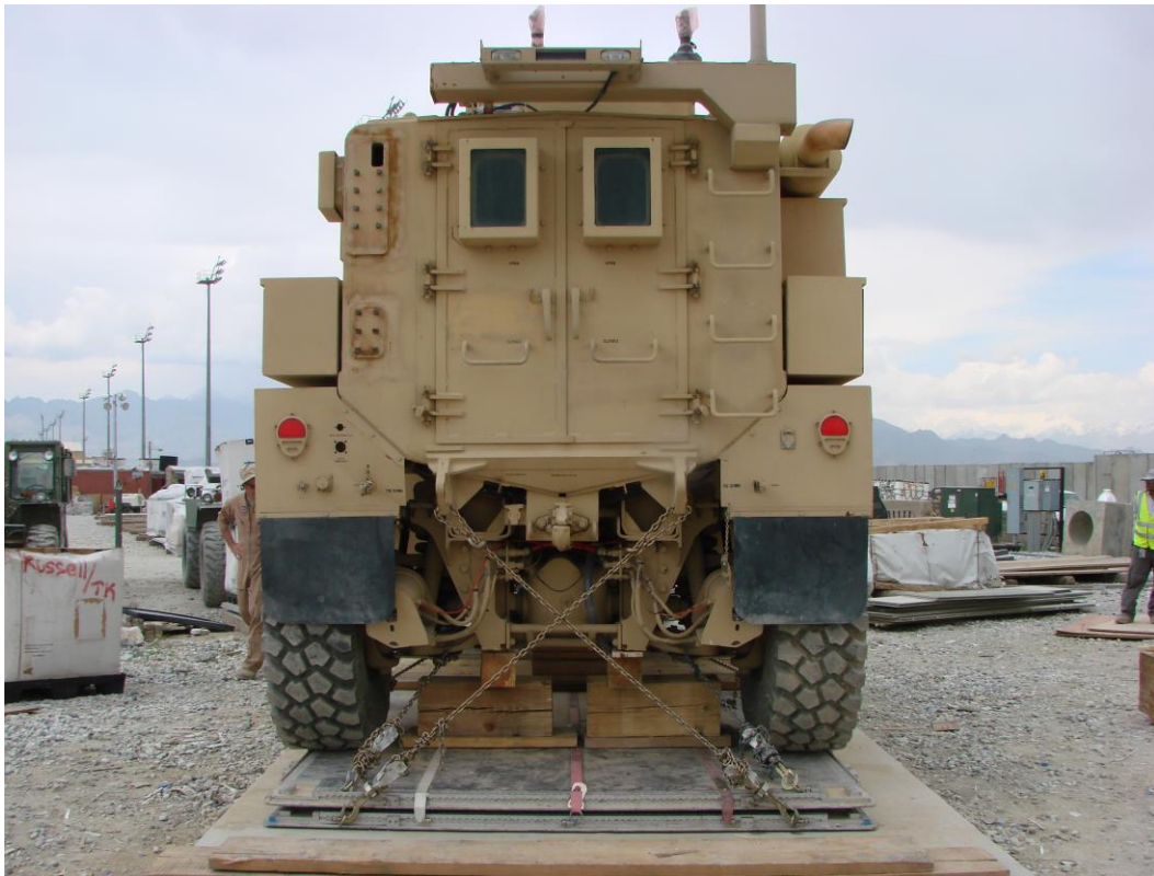
Photo 9: Photo of shoring demonstration of a 18-ton Cougar (aft view).
