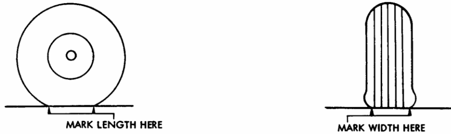
Figure 6-18. Measurement of Tire Footprint
