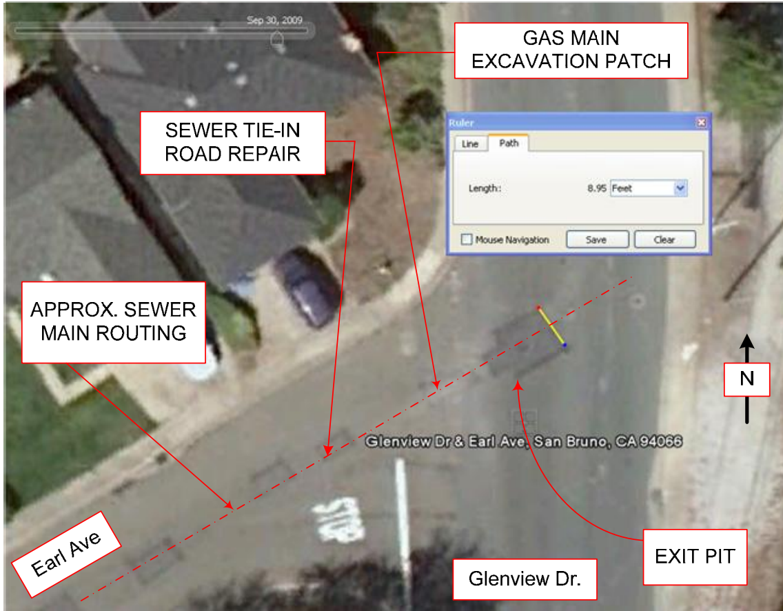
Figure 8: Google Maps and Paving Patches Post 2008 Sewer Repair
