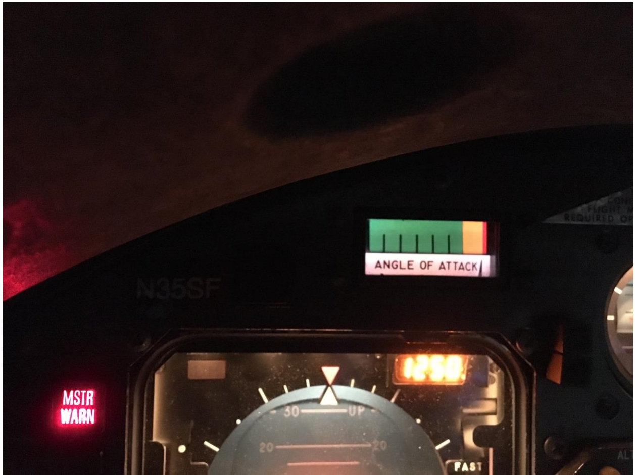
Photo 4: Close of AOA gauge with Master Caution light illuminated.
