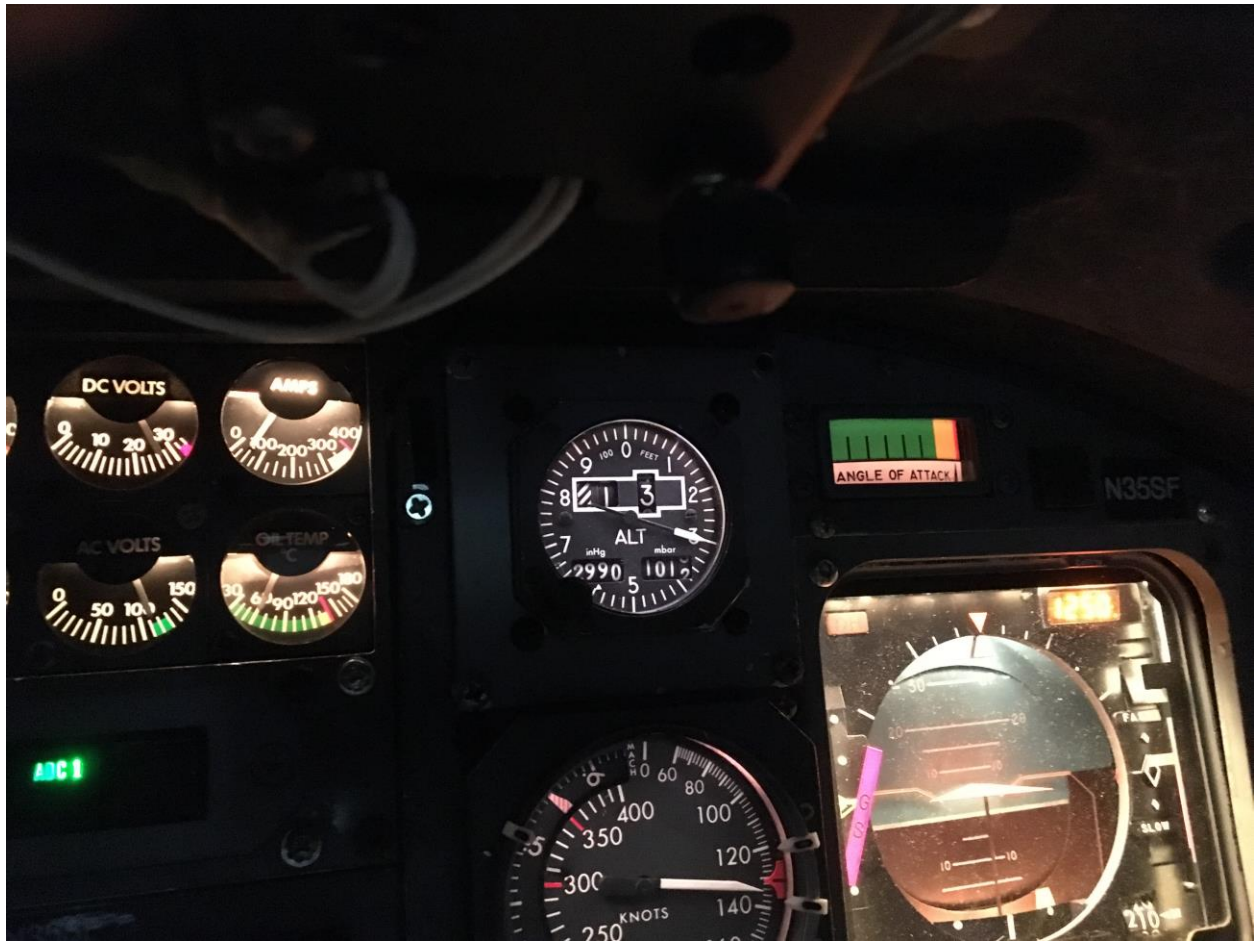
Photo 2: Captain's instrument panel with AOA gauge.
