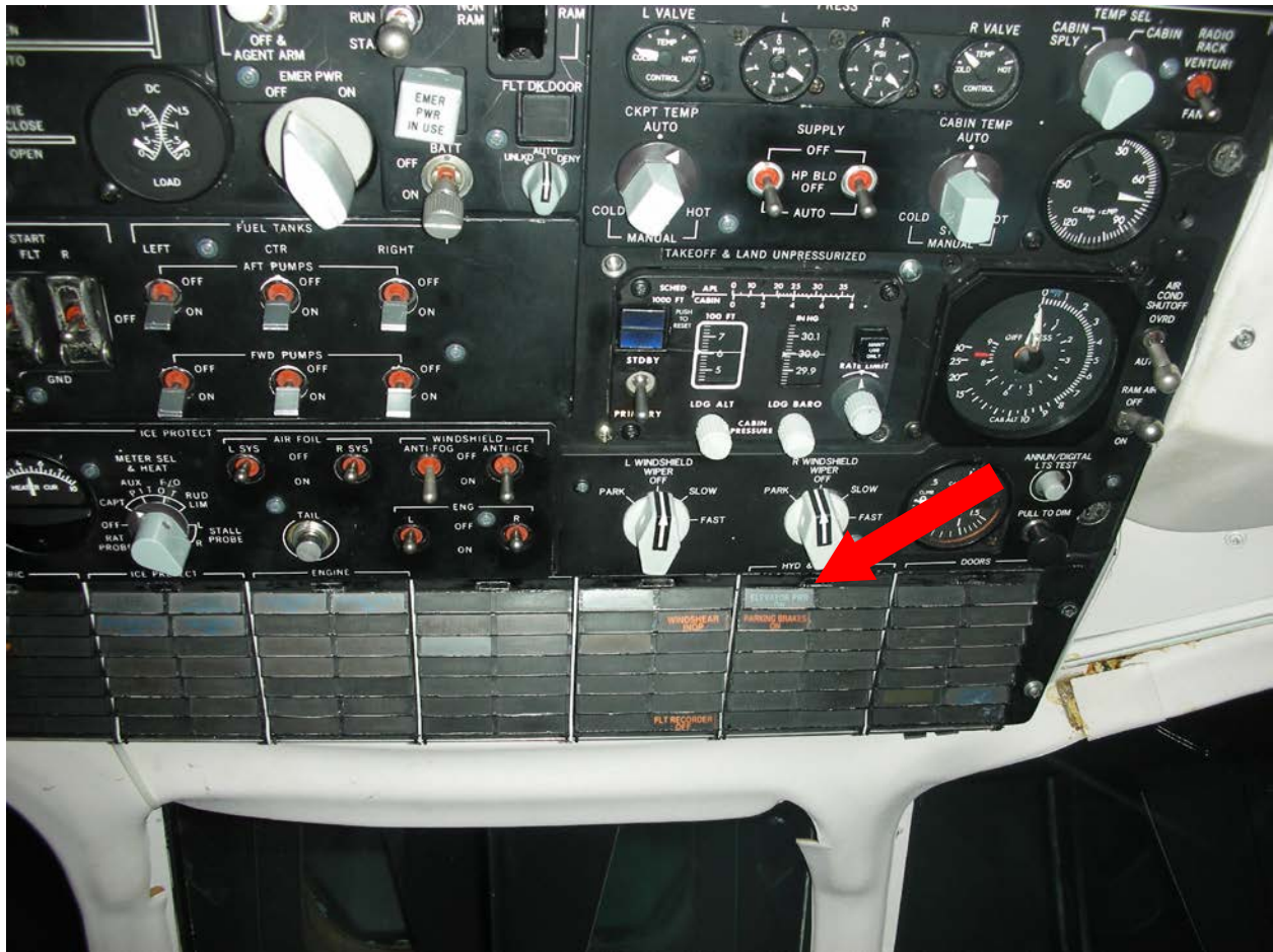
Photo 5: Overhead annunciator indications with control column full forward. “Elevator Pwr On” light indicated by arrow.
