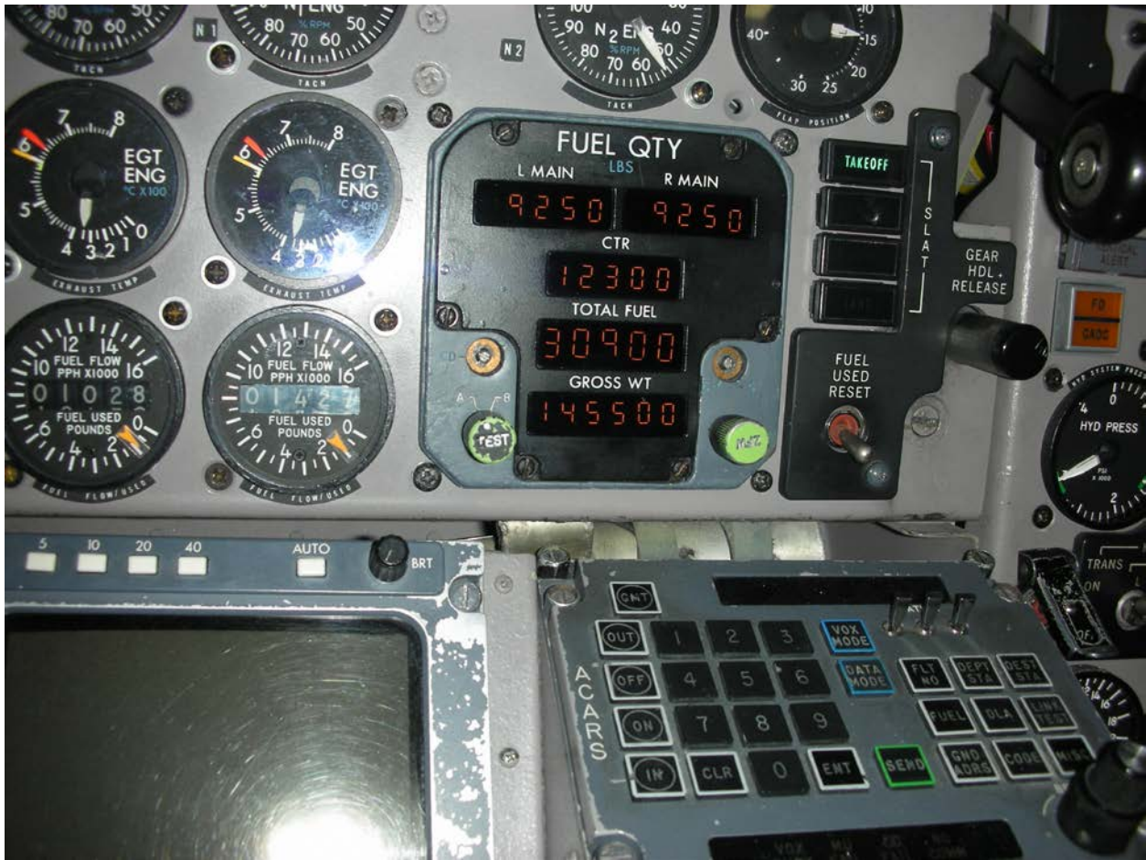
Photo 2: Fuel panel indications.
