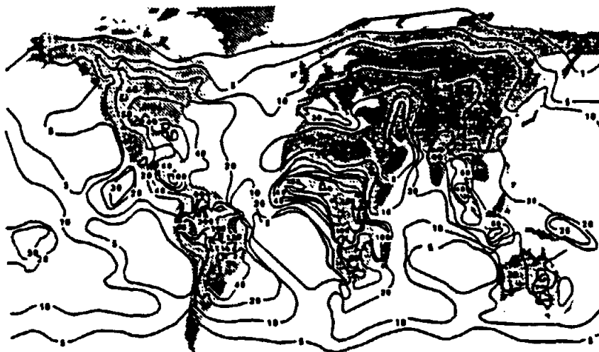
Figure 4. Average annual worldwide thunderstorm days. Note that the highest windshear threat occurs in the tropics.
