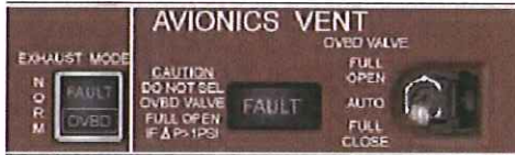
Avionic vent panel with overboard valve on full close
