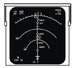
It must be remembered that the displayed TOD point is calculated based upon the FMC entered wind entries, cruise altitude, descent/speed constraints and cost index. Should any of these conditions change significantly without being entered into the FMC, the TOD point may be inaccurate. Although the FMC will normally calculate an adequate distance to begin the descent from the cruise altitude, it should not be used as a substitute for good mental planning.
