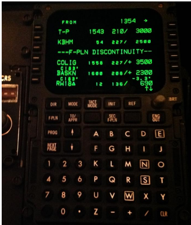
Photo 11: CDU F-PLN page with approach not sequenced. 141
