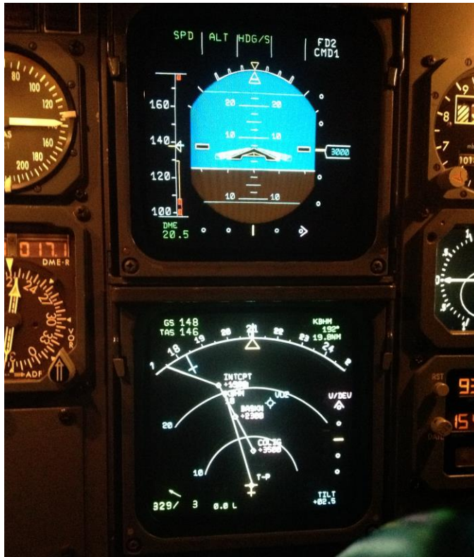
Photo 10: PFD/ND with approach not sequenced. 140
