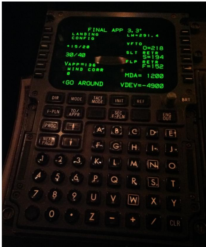
Photo 7: CDU after activating Final Approach Mode 131
