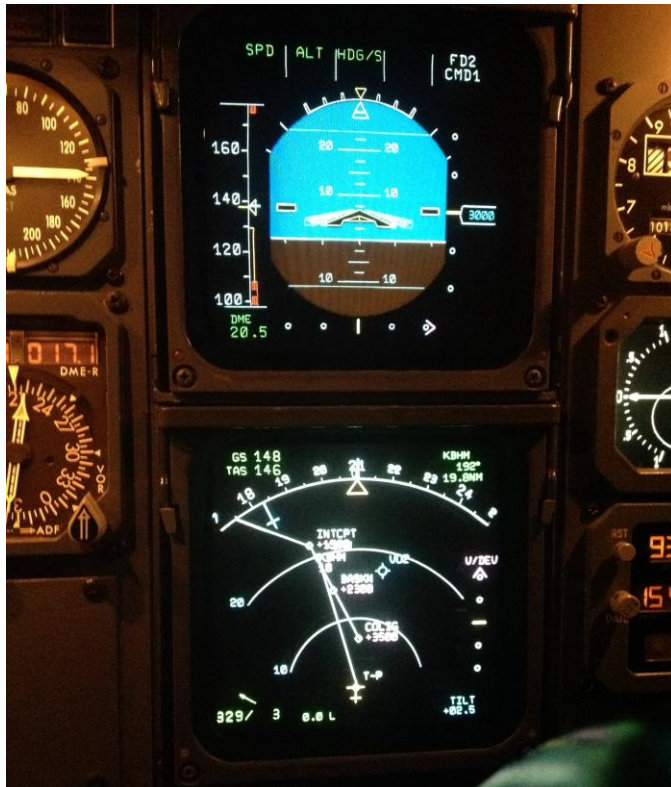
Photo 5: PFD and ND with flight plan route discontinuity in the active flight plan. 128
