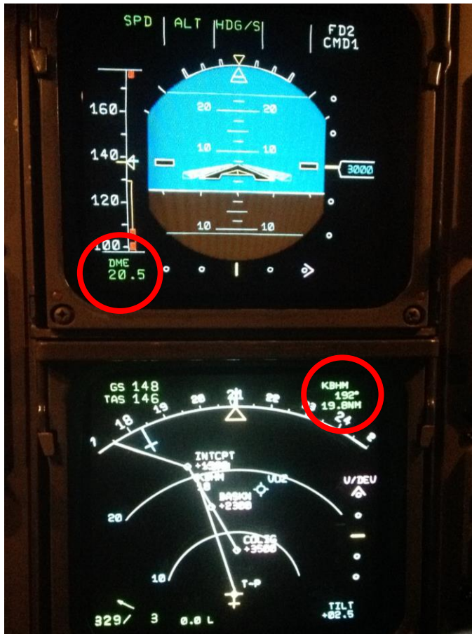
Photo 3: PFD (top screen) showing localizer DME. Bottom screen (ND) showing next waypoint distance. 122
