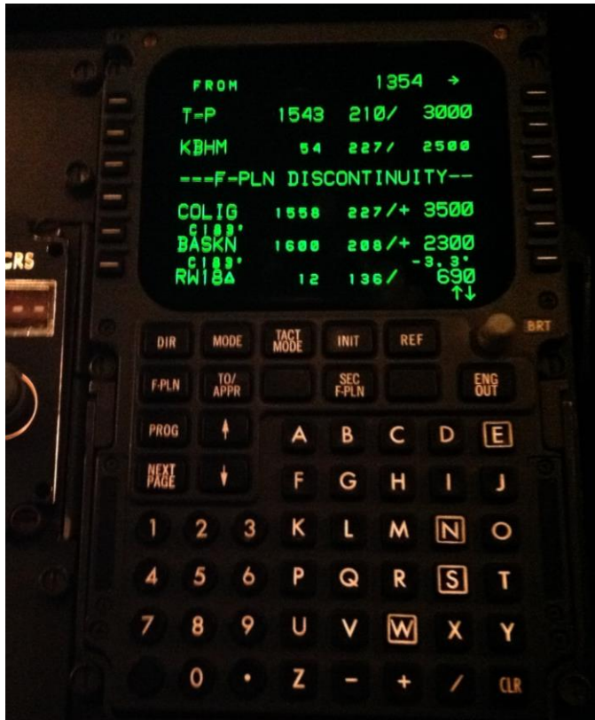
Photo 4: CDU F-PLN page showing flight plan discontinuity. 127
