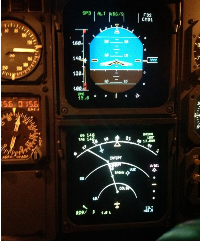
Photo 9: PFD and ND with re-sequenced flight plan. 138
