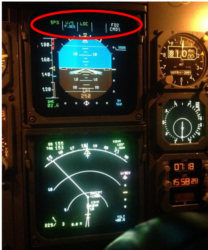
Photo 2: Photo of the Primary Flight Display PFD (top screen) and Navigational Display (bottom screen). The FMA is indicated by circle. 112
