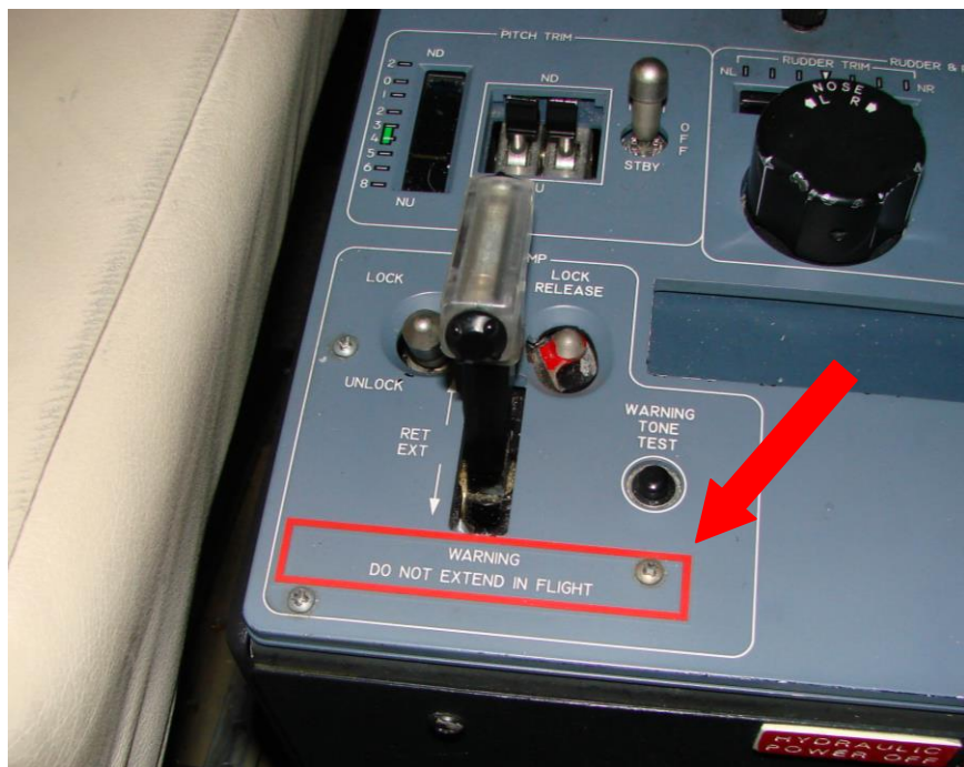
Photo 16: Lift dump required placard 124
