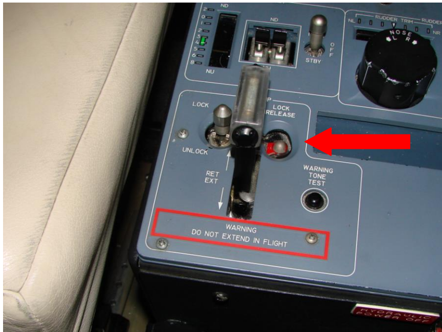
Photo 13: Lift dump handle in the locked position (arrow points to mechanical LOCK RELEASE button) 119
