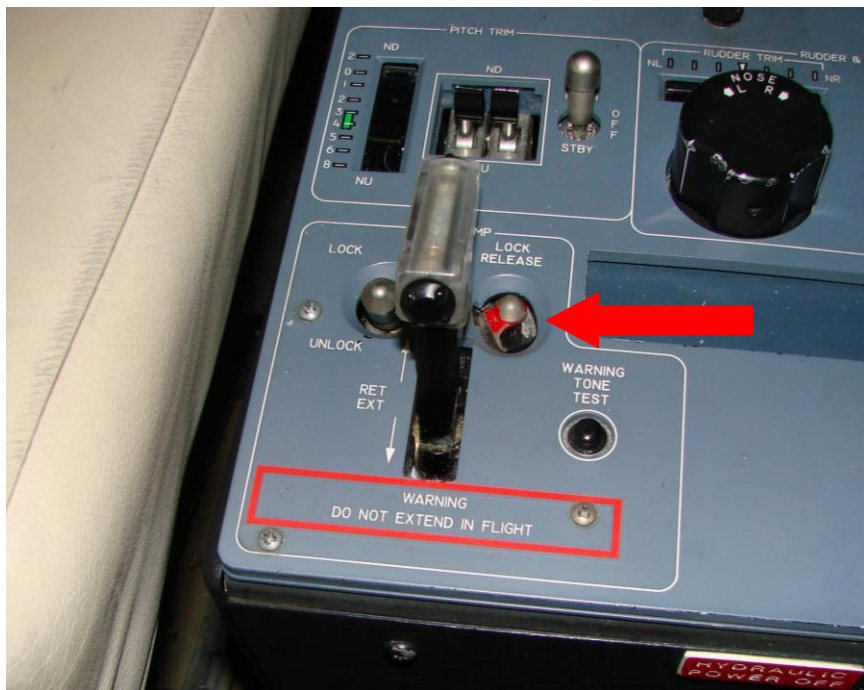
Photo 14: Lift dump handle in the unlocked position (arrow points to mechanical LOCK RELEASE button) 120
