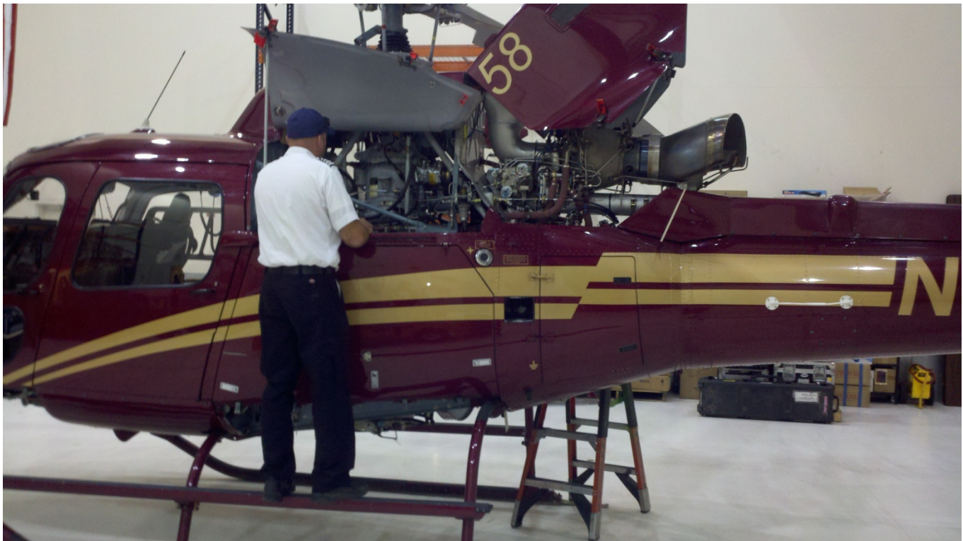
Pilot conducting a preflight inspection of the left MGB area
