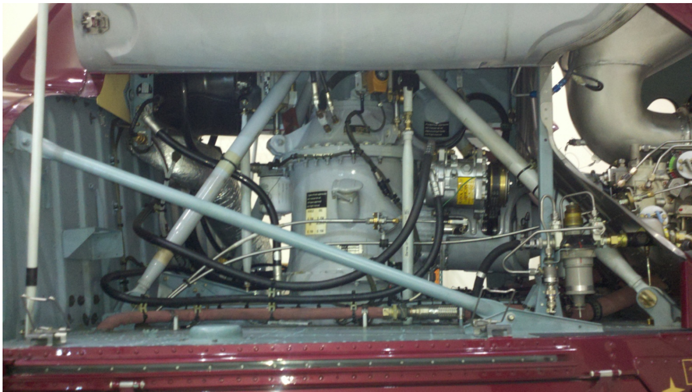
Left MGB inspection area
