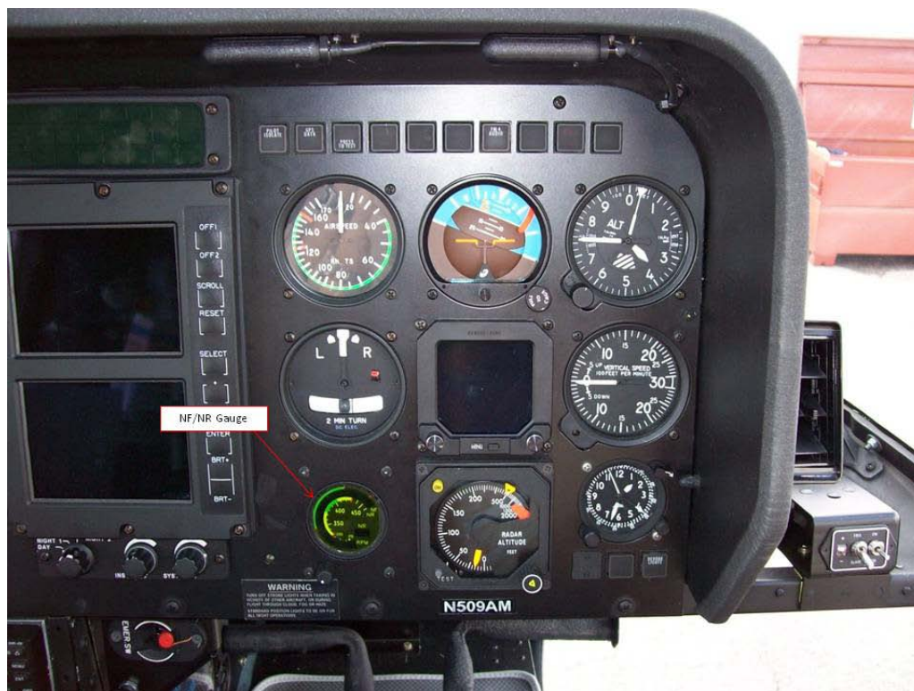
Fig 3 - N509AM pilot instrument panel. Location of the NF/NR gauge indicated by the red arrow.
