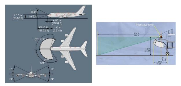
The A-380 Flight Crew binocular vision chart<sup>22</sup> below indicates that as the Air France A-380 airplane was making the turn onto Taxiway Alpha, a 10 degree cone of vision may have blocked
