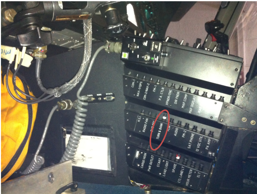
Figure 7. Photograph of the helicopter’s circuit breaker panel taken on June 18, 2012. The circuit breaker for the turn and bank indicator is in the off position (pulled out).
