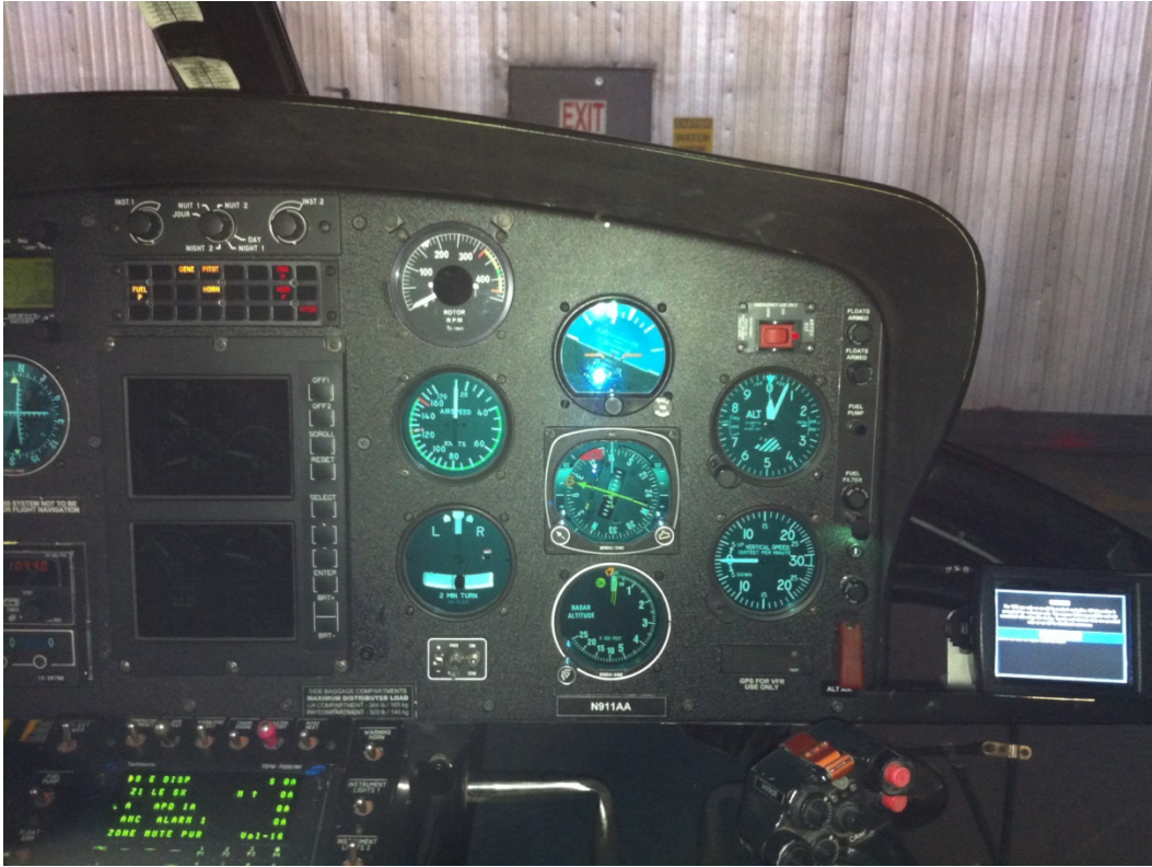
Figure 6. Photograph of the right side of the helicopter’s instrument panel taken on June 18, 2012. The small screen on the lower right side of the photograph is the Garmin 296 GPS unit.
