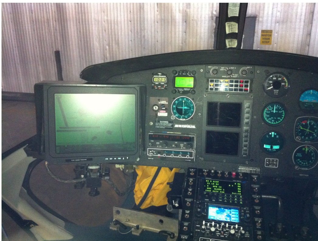
Figure 8. Photograph of the left side of the helicopter's instrument panel taken on June 18, 2012. The large screen on the left side of the photograph is the Avalex mapping system display screen. The lighted screen in the lower center of the photograph is the Garmin GNS-430.
