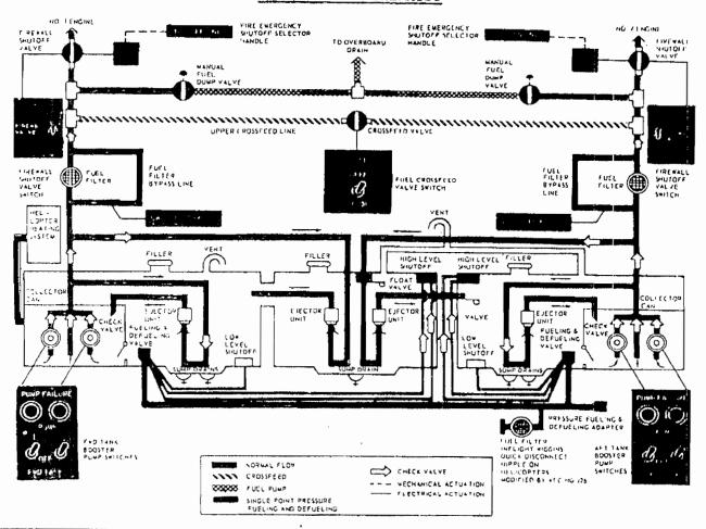
This helicopter is equipped with a three tank fuel system. During normal operations the forward tank provides fuel for the No. 1 engine, the aft tank provides fuel for the No. 2 engine, and the center tank replenishes consumed fuel through the ejector system. Transfer of fuel to the aft tank through the ejector system is prevented by float valve actuation until approximately 550 pounds of fuel remains in the center tank.
