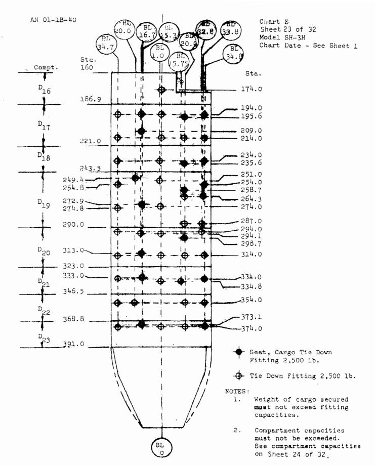
NOTICE: Cargo tie down data on this page are only applicable to aircraft equipped with NARP Airframe Change No. 316.
