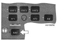
**Note:** When standby tuning is desired, the NAV keys on both RMPs (if operable) are selected on. The STBY NAV keys then become operative.
