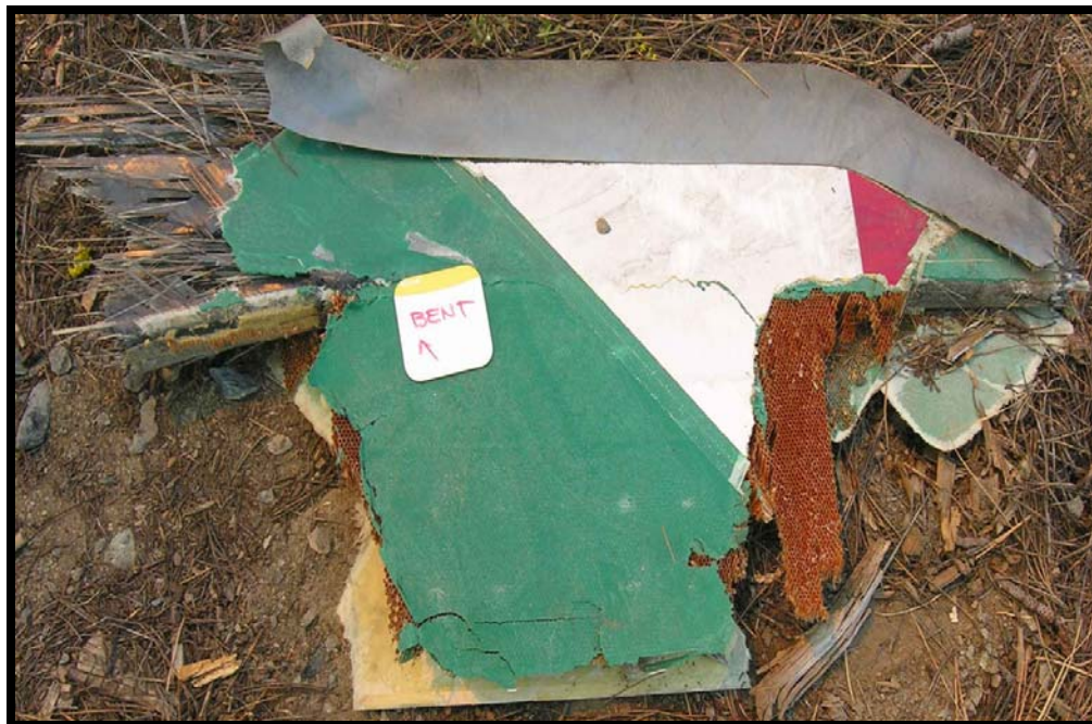
Figure 06: Outboard section of rotor blade (see figure 05 for location found)
