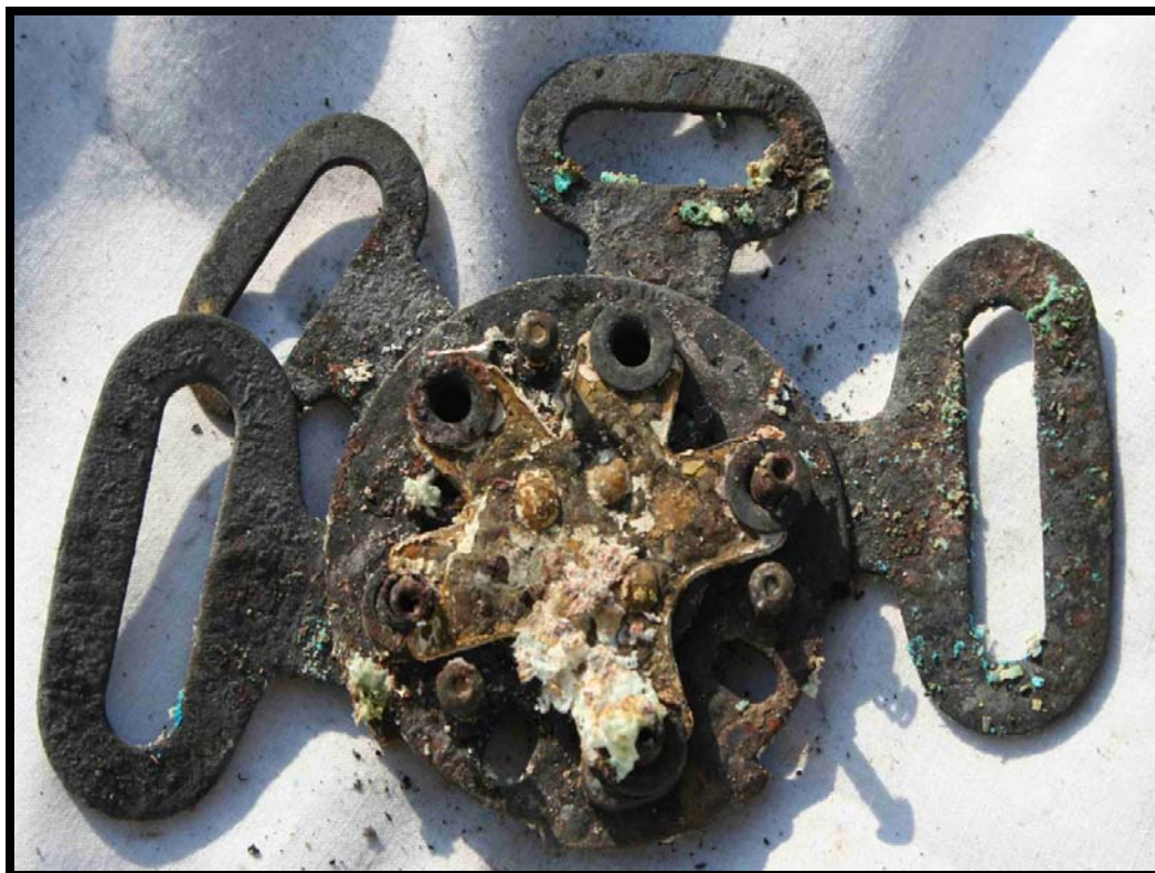
Figure 22: Engaged seatbelt buckle (all found were engaged)
