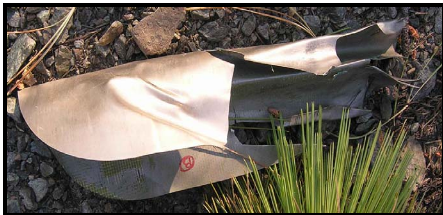
Figure 10: Main rotor blade tip found below first tree cut
