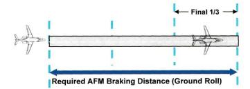
Clearly, in order to achieve AFM landing distance performance, the pilot must depend upon the anti-skid power brake system. Pilot perception of the stopping performance of the airplane must be balanced by proper understanding of the operating characteristics of the airplane.
