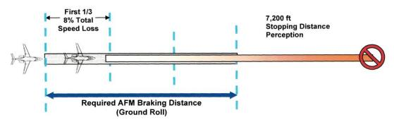
As the airplane enters the middle 1/3 of the braking distance, the deceleration rate increases, resulting in a speed reduction to about 59% of the touchdown speed. The perceived stopping distance, although shorter now, may still appear to be in excess of the available runway.
