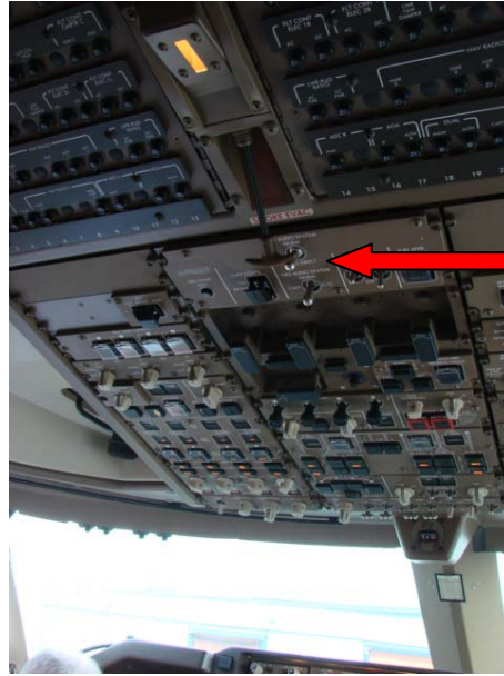
Figure 6: Smoke Evacuation Handle (pulled)
