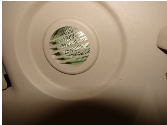
Figure 8: Smoke Evacuation Port (cockpit ceiling)
