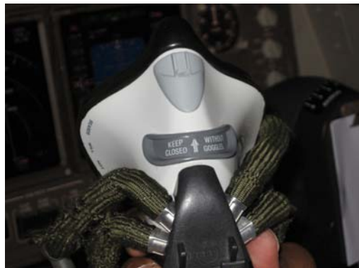
Figure 9: Smoke vent valve selector (closed) Figure 10: Smoke vent valve selector (open)
