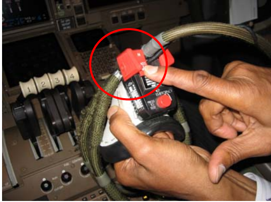
Figure 14: 100% Selector Switch on Oxygen Mask
