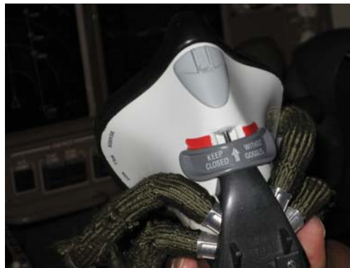
Figure 9: Smoke vent valve selector (closed) Figure 10: Smoke vent valve selector (open)
