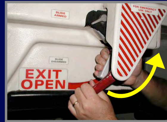
3. While holding Slide Arming handle in the aft position – pull Emergency Door Control Handle aft and upward. (Red Handle)
