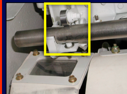
Girt Bar installation in the bottom of the Cabin Door
