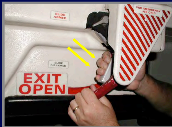
2. Pull slide arming handle aft more.
