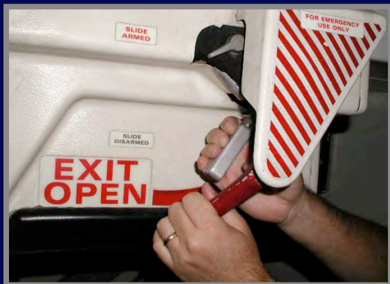
1. Pull slide arming handle aft.
