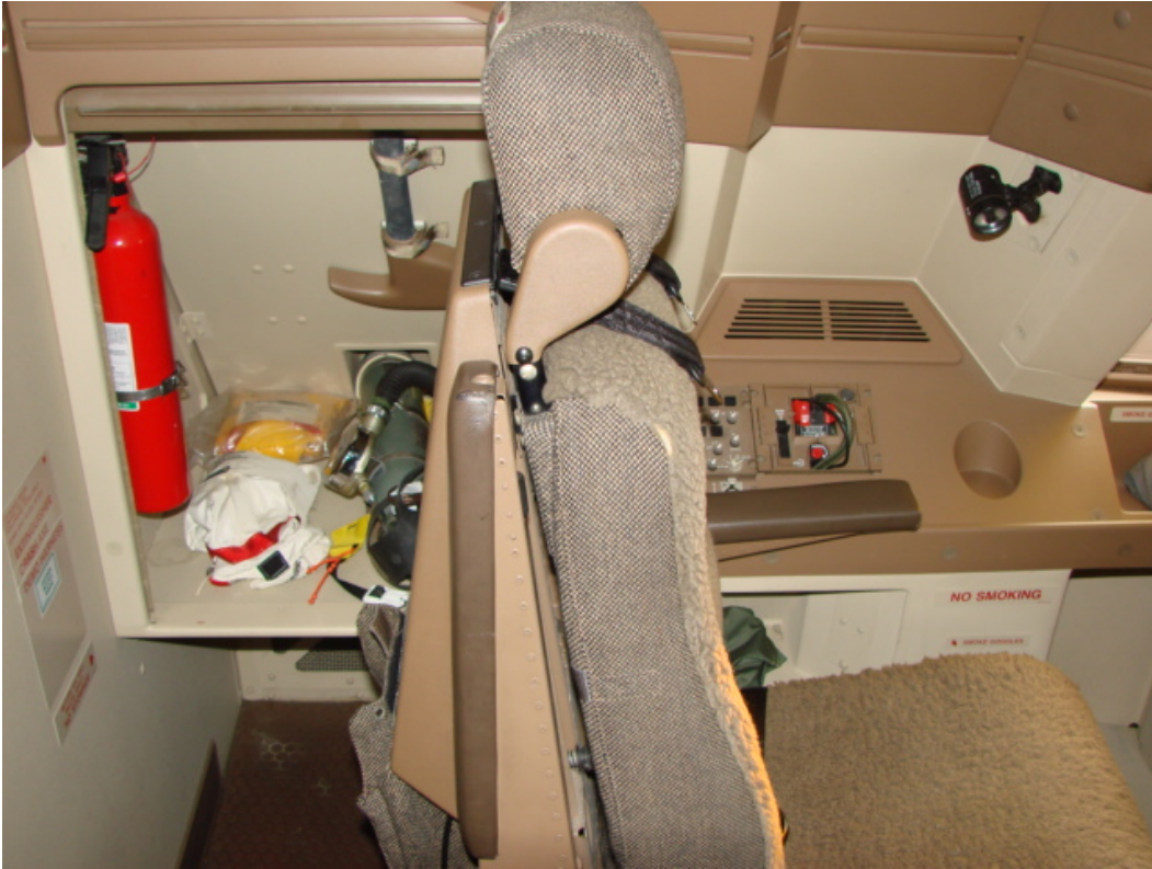
Photo 18 Left observers' seat w/ emergency equipment closet
