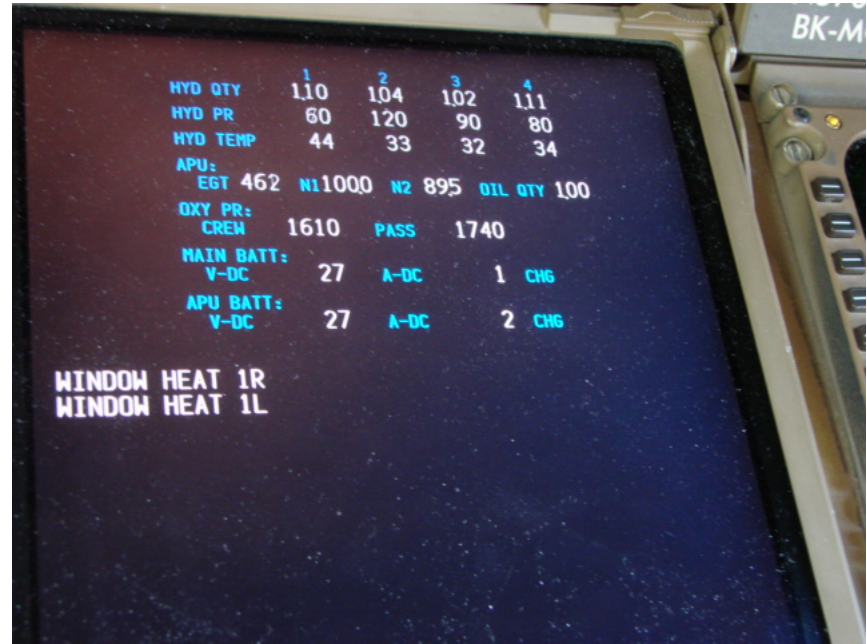
Photo 16 Oxygen synoptic page (note oxygen pressure)
