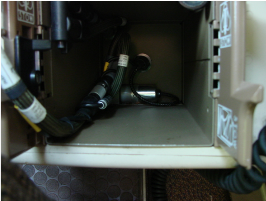
Photo 15 Pressure switch in cockpit oxygen mask box
