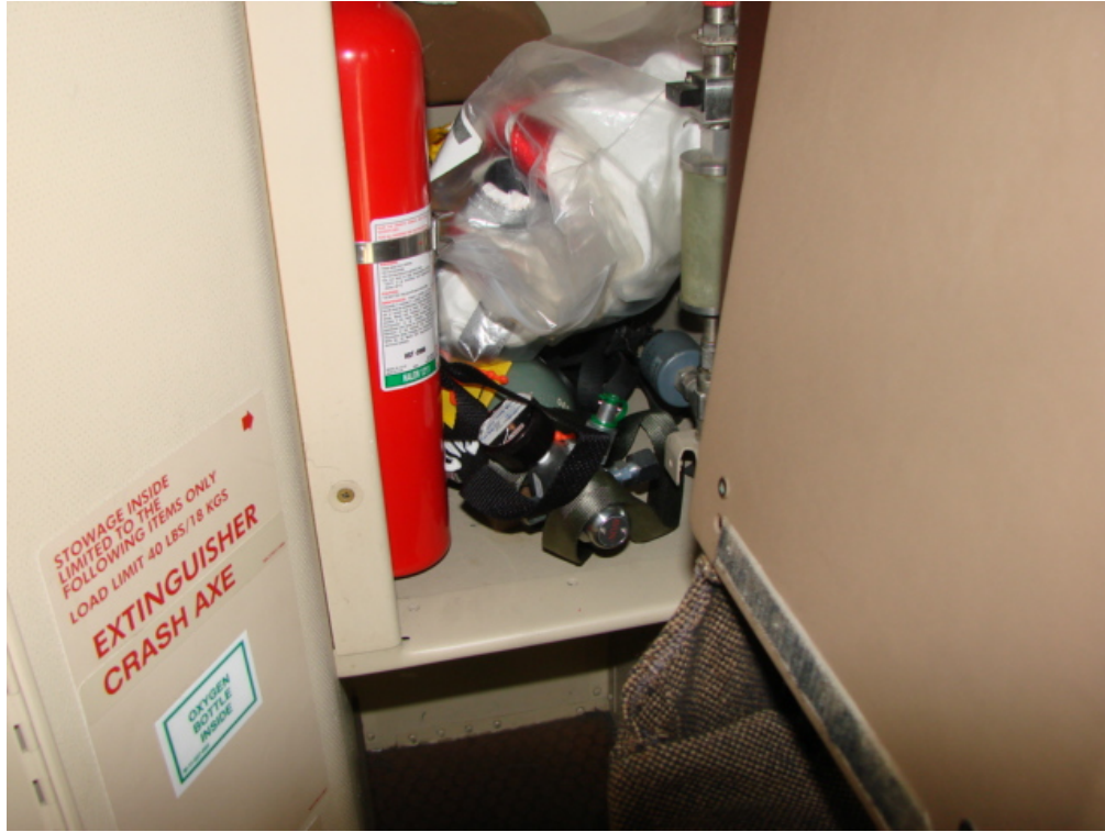
Photo 10 B747-400BCF emergency equipment cabinet
