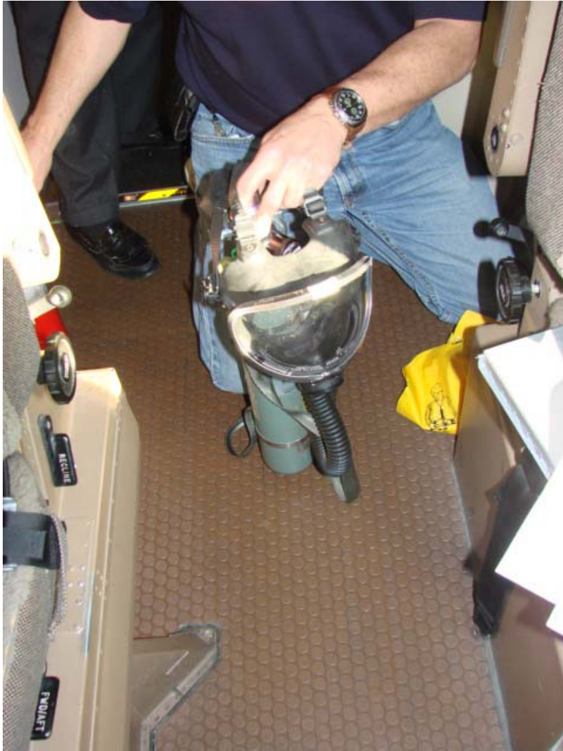
Photo 12 B747-400BCF portable O2 bottle (removed)
