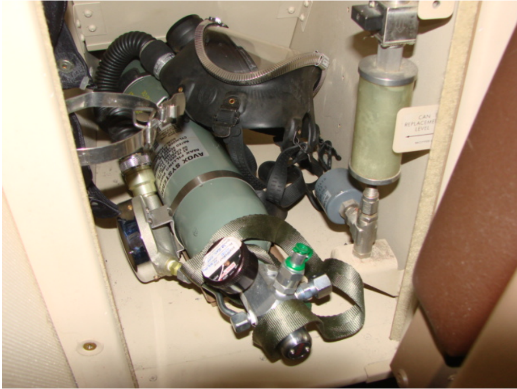
Photo 11 BCF portable cockpit O2 bottle (Halon bottle removed)
