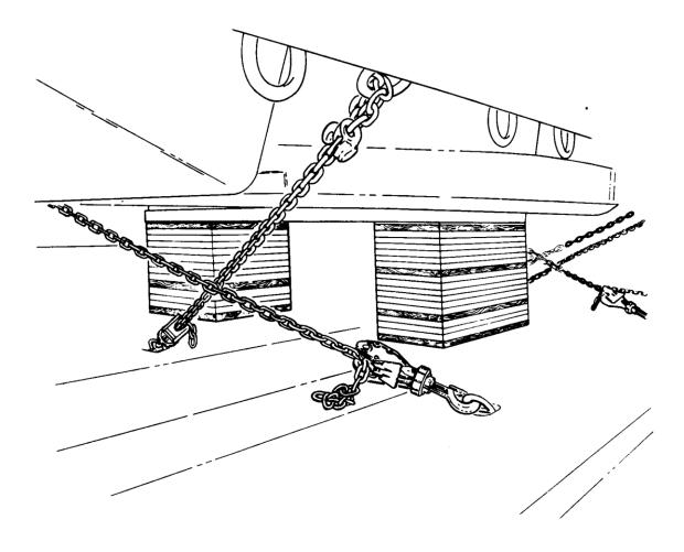
Note: While loading the Strikers the straps should not be completely tighten. By over tighten the straps the 20 Ft pallet may become bowed causing the PDU to lose traction and preventing the pallet to move. Over the pallet is in position, all straps must be tighten again to prevent the vehicle from moving in flight
