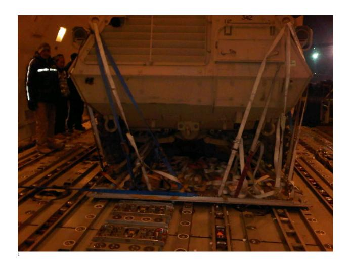
To prepare the Striker Vehicles we will have to build the vehicles on sleeper onto the 20 Ft pallet. The vehicle should be placed on top of sleeper shoring similar to the shoring shown in the picture below.
