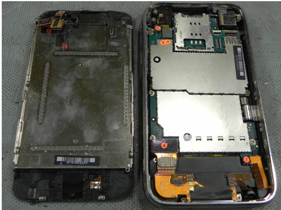
Figure 2. Internal inspection of Apple iPhone 3GS.
