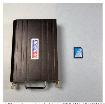
Figure 2. The HDD and SD card associated with the MDR (SN: 1508MCU80013) from the SD54.
