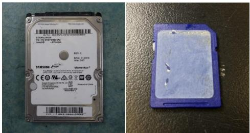
Figure 1. The HDD and SD card associated with the MDR (SN: 1603MCU80040) from SD7. The HDD has been removed from the MDR enclosure in this photograph (left).
