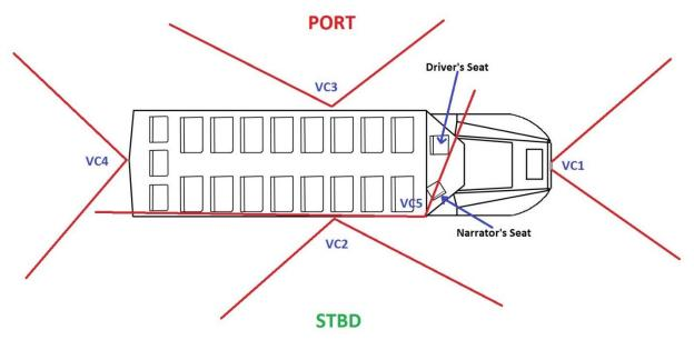
Figure 5. A top down view of a DUKW showing the layout of the camera locations and their approximate field of view for SD7, SD54, SD27 and SD17.
