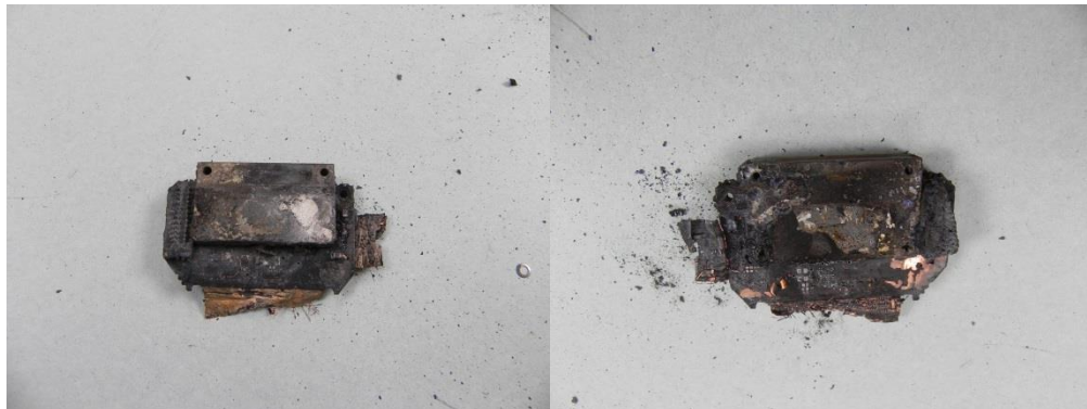
Figure 3. The front (left) and rear (right) of the internally mounted NVM chassis.
