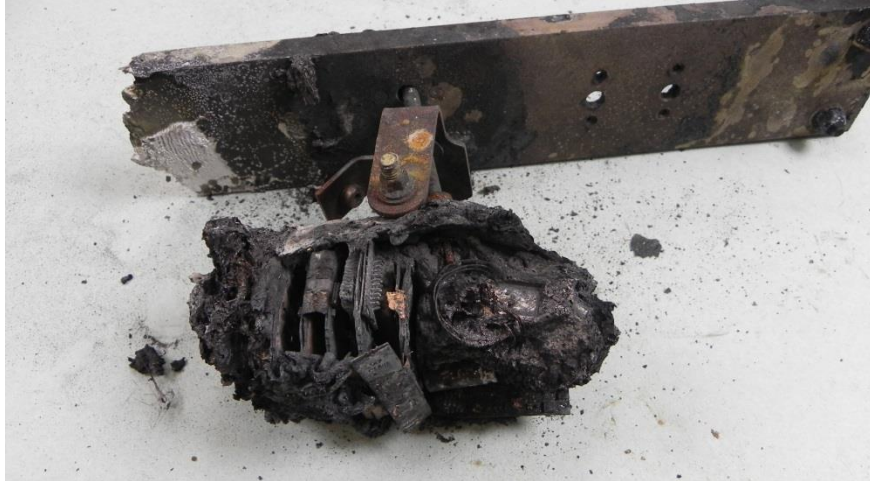
Figure 1. The arrival condition of the Appareo Vision 1000.
