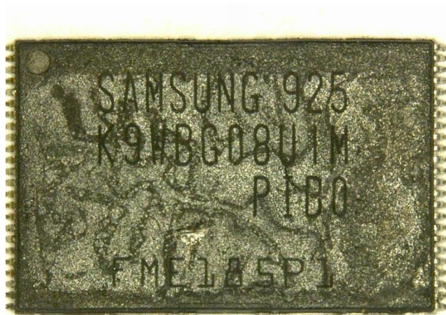
Figure 7. Bubbling along NVM chip 2's surface indicative of high temperature heat damage.
