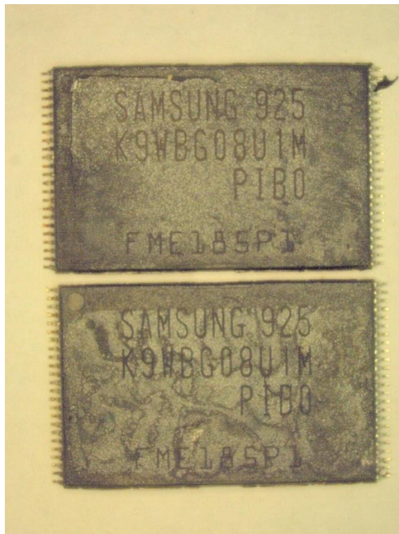
Figure 5. The two individual internal NVM chips after removal and cleaning.
