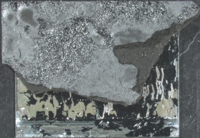
2 mm Appereo-SD-5 segment 1; broken SD package, front view
