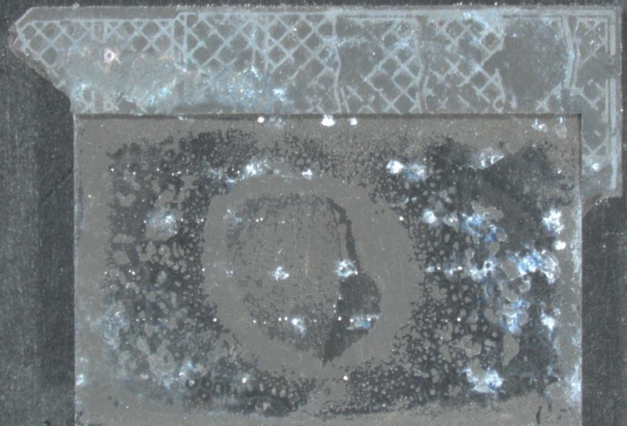
2 mm Appereo-SD-5 segment 1; broken SD package, back view
