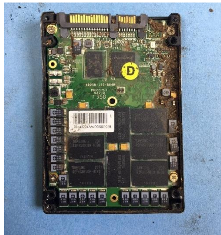
Figure 2. The SSD with the outer casing removed.
