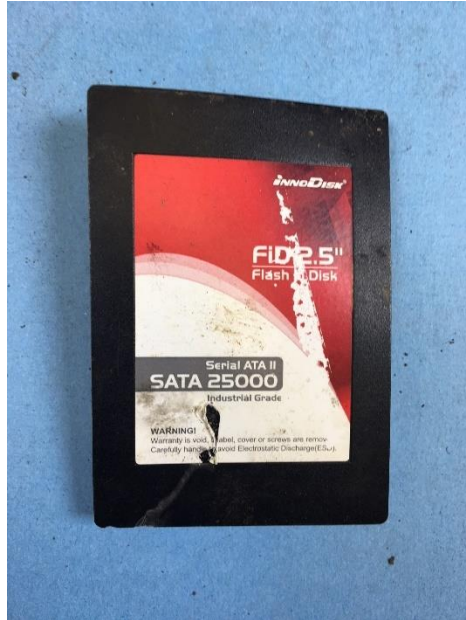
Figure 1. The condition of the SSD's outer casing.
