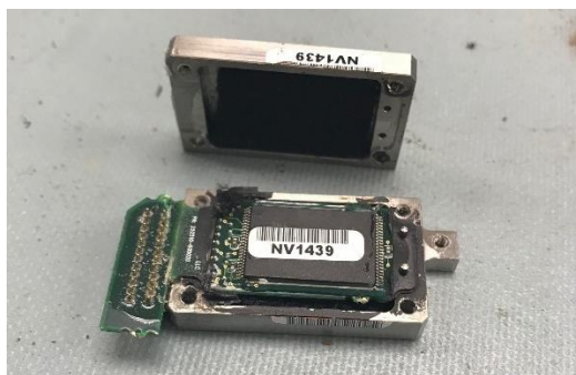
Figure 2. The internal NVM as it was extracted from the device.
