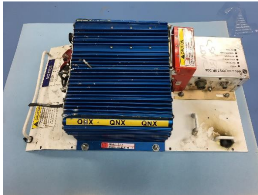
Figure 2. The Wabtec VideoTrax recovered from AMTK47.
