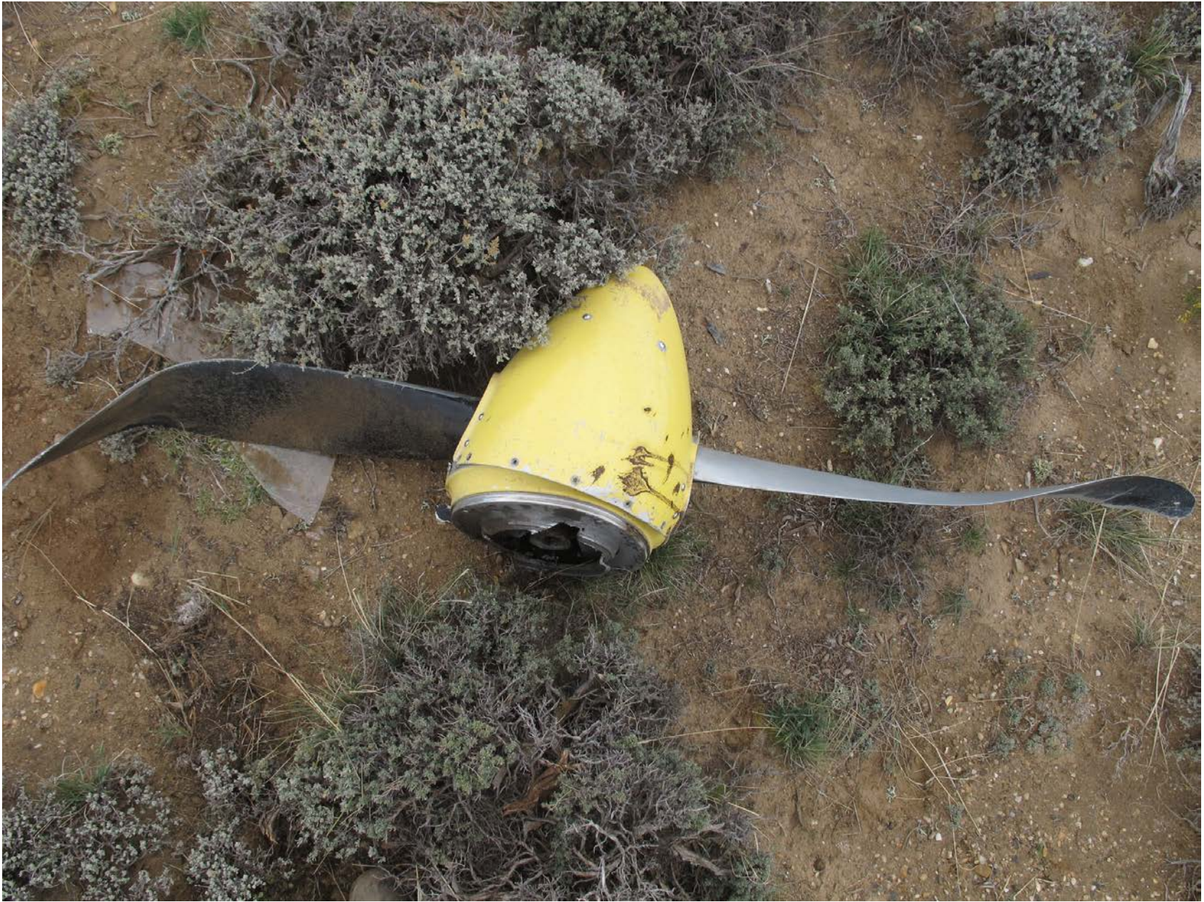
Photo 5 – Propeller exhibiting blade twisting.
