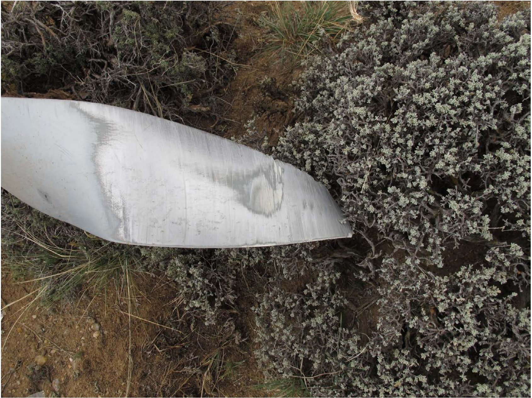
Photo 6 – Propeller blade showing chordwise scratches and polishing.
