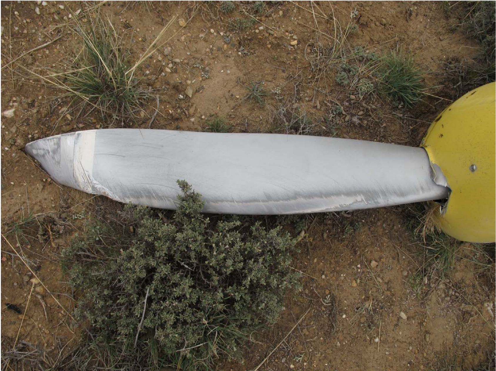
Photo 7 – Propeller blade showing leading edge damage and polishing.
