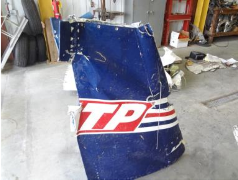
Photo 19: Right Side View of Vertical Stabilizer
