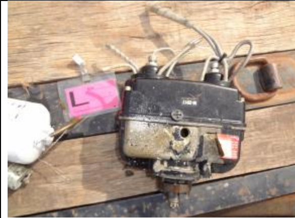
Photo 7: Left Magneto - Post Recovery
