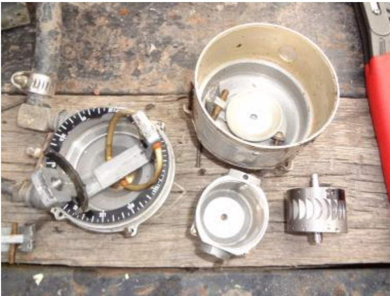
Photo 4: HSI - Post Disassembly
