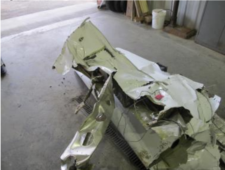
Photo 5: Left Wing - Post Recovery (Courtesy of Piper Aircraft)
