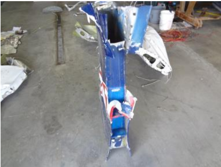
Photo 18: Aft View of Vertical Stabilizer (Devoid of Rudder)
