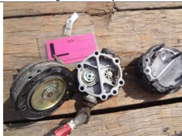
Photo 12: Left Engine Driven Fuel Pump - Post Disassembly
