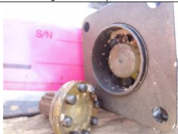
Photo 10: Left Engine Vacuum Pump with Sheered Shaft
