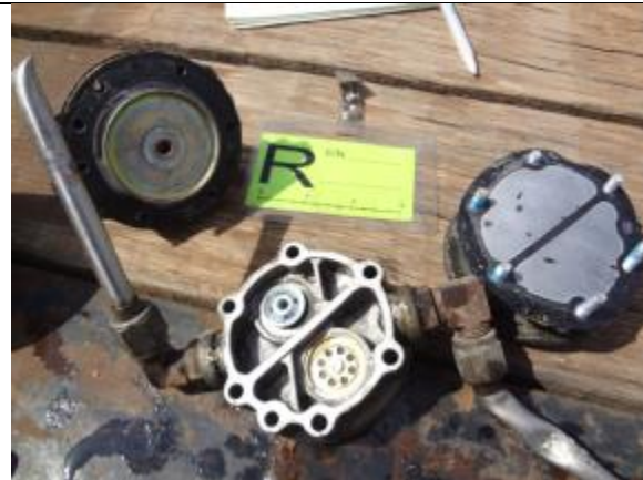
Photo 25: Engine Driven Fuel Pump - Post Disassembly
