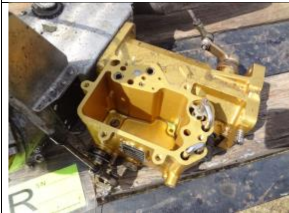
Photo 26: Right Engine Carburetor with Fuel Present - Post Disassembly
