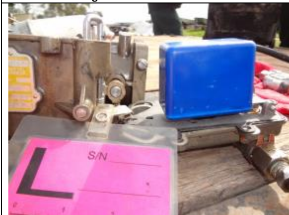
Photo 15: Left Engine Carburetor Float Assembly - Post Disassembly
