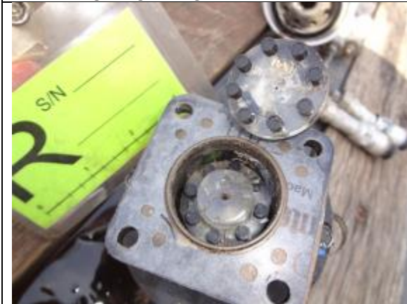
Photo 24: Right Vacuum Pump with Sheered Shaft – as Viewed Post Removal
