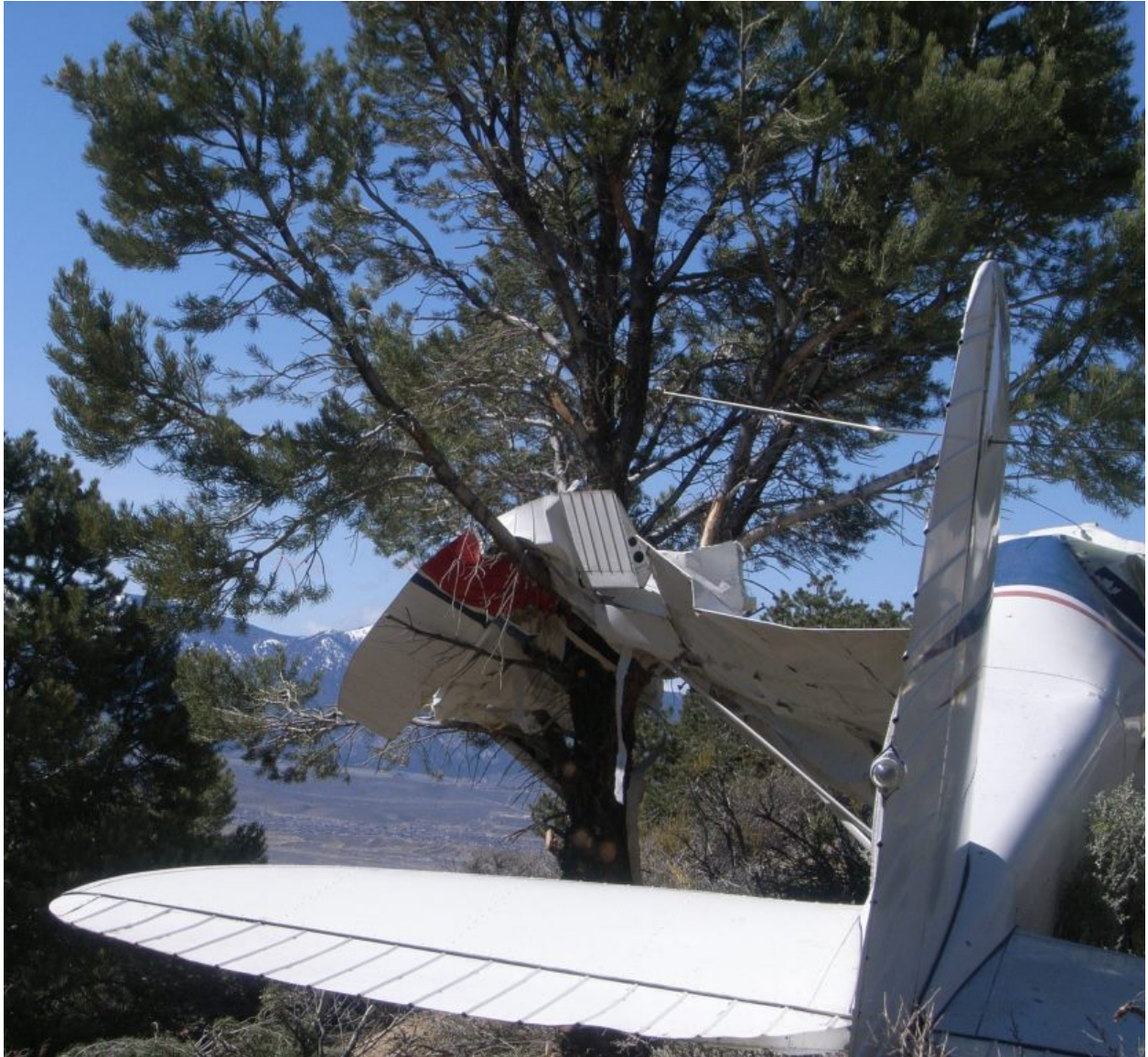
Figure 5 – Empennage and Left Wing in Tree (Note undamaged branches)
