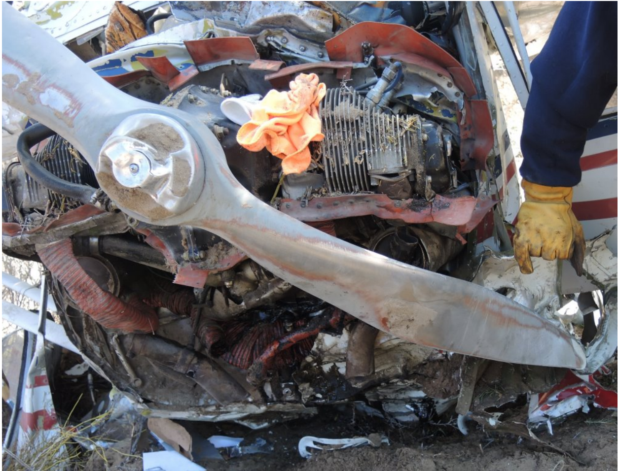
Figure 24 – Bent Propeller Blade (Note scouring)
