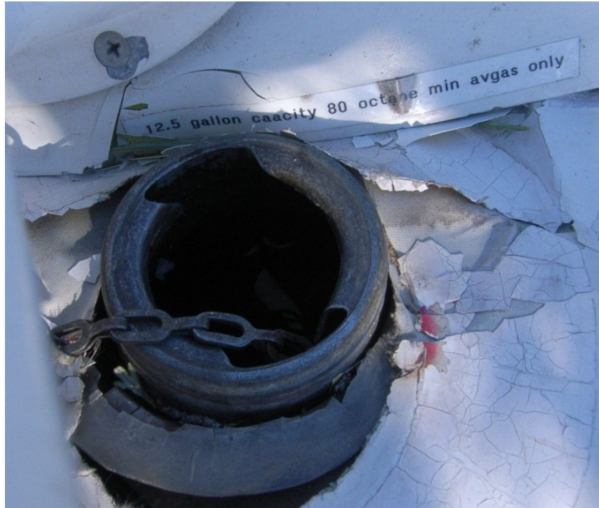
Figure 10 - Fuel Filler Neck with Placard (Cap removed by investigators)
