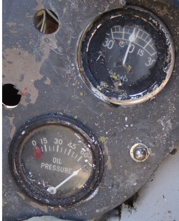
Figure 13 - Ammeter and Oil Pressure Indicators
